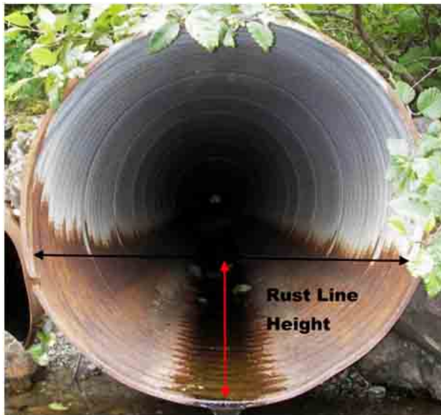
Figure 14a.—Photograph illustration of rust line height.
