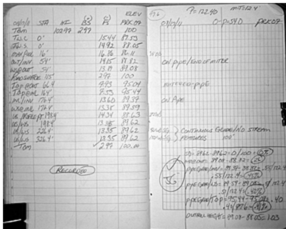
Figure 45.—Sample of survey data and calculation in a field notebook.
