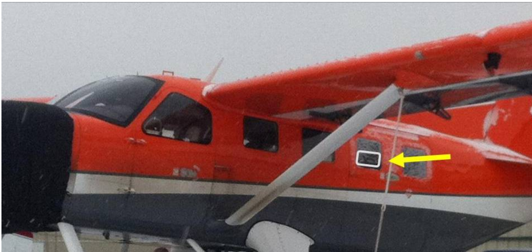
Figure 2. Quest Kodiak-100 survey aircraft used on the fall molt survey of Steller’s eiders along the Alaska Peninsula in 2012. The arrow points to the second to last window on the left (port) side of the aircraft through which photographs were taken. A simulated model of a rectangular window port (indicated by a yellow arrow) would allow the photographer to pan and shoot through an open window, decreasing plexiglas image distortion. The port would be hinged at its bottom edge and could be opened and closed during flight. (See the pre-existing port near the front of the pilot’s side window, as an example).
