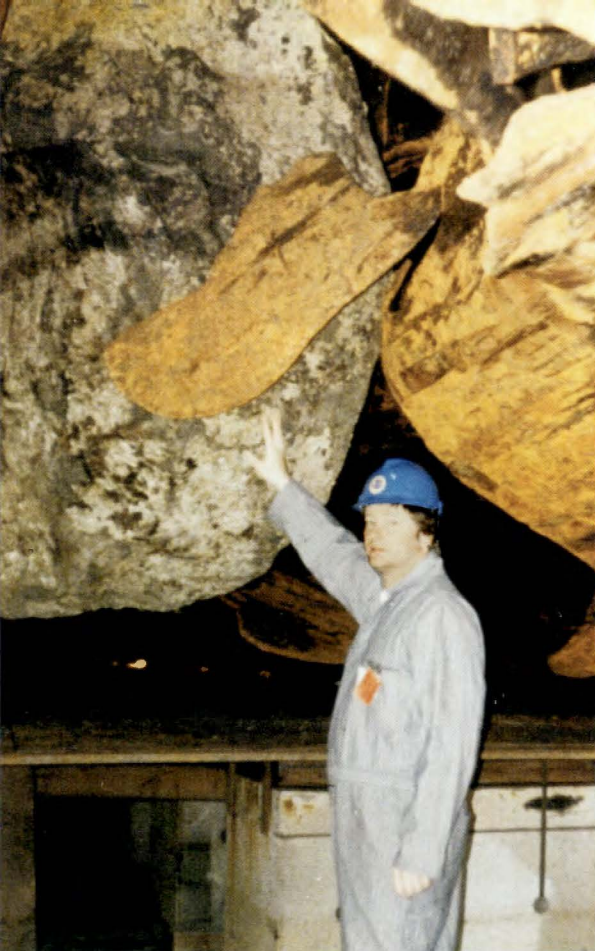
Craig Tillery inspects a boulder-sized piece of Bligh Reef caught in the torn hull of the Exxon Valdez tanker.
