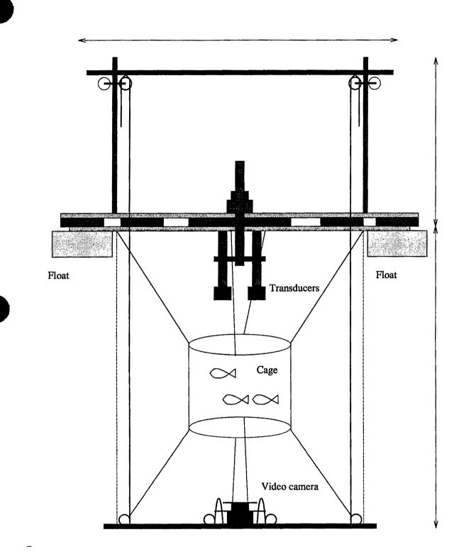
Figure 7. Preliminary design of fish support apparatus
