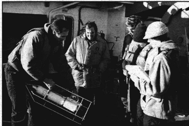
Dr. Carl Schoch shows oceanography students how a CTD records information as it descends to the bottom of the ocean.
