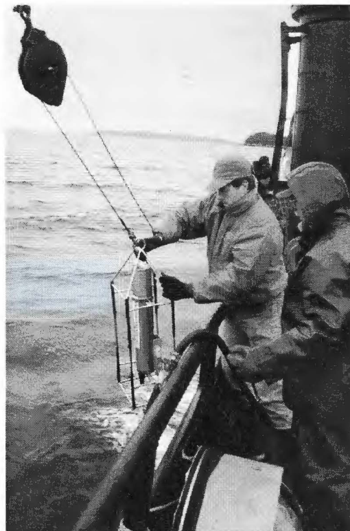
Jim Murphy hauls in a CTD (current/temperature/depth) recorder while Dr. Ted Cooney looks on. The SEA program surveys collected nearly 1,000 CTD measurements during the 1994 field season. Photo by Robert Spies.
