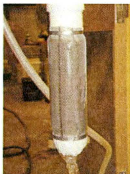
Figure 5: Left panel. The screen that covers the tip of the injection well (length of screen is approximately 0.30 m long, a foot). Right panel: Photograph of the HPI at Beach 1 (Figure 1). Copyright Groundwater Monitoring and Remediation, From Boufadel and Bobo (2011).
