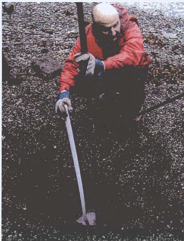
Figure 1: Placement of PVC pipe (white) for measurement of water level and multiport sampling well (stainless steel) in a pit. This approach would be used to monitor the background concentration of oxygen and nutrient in the lower layer of beaches.
