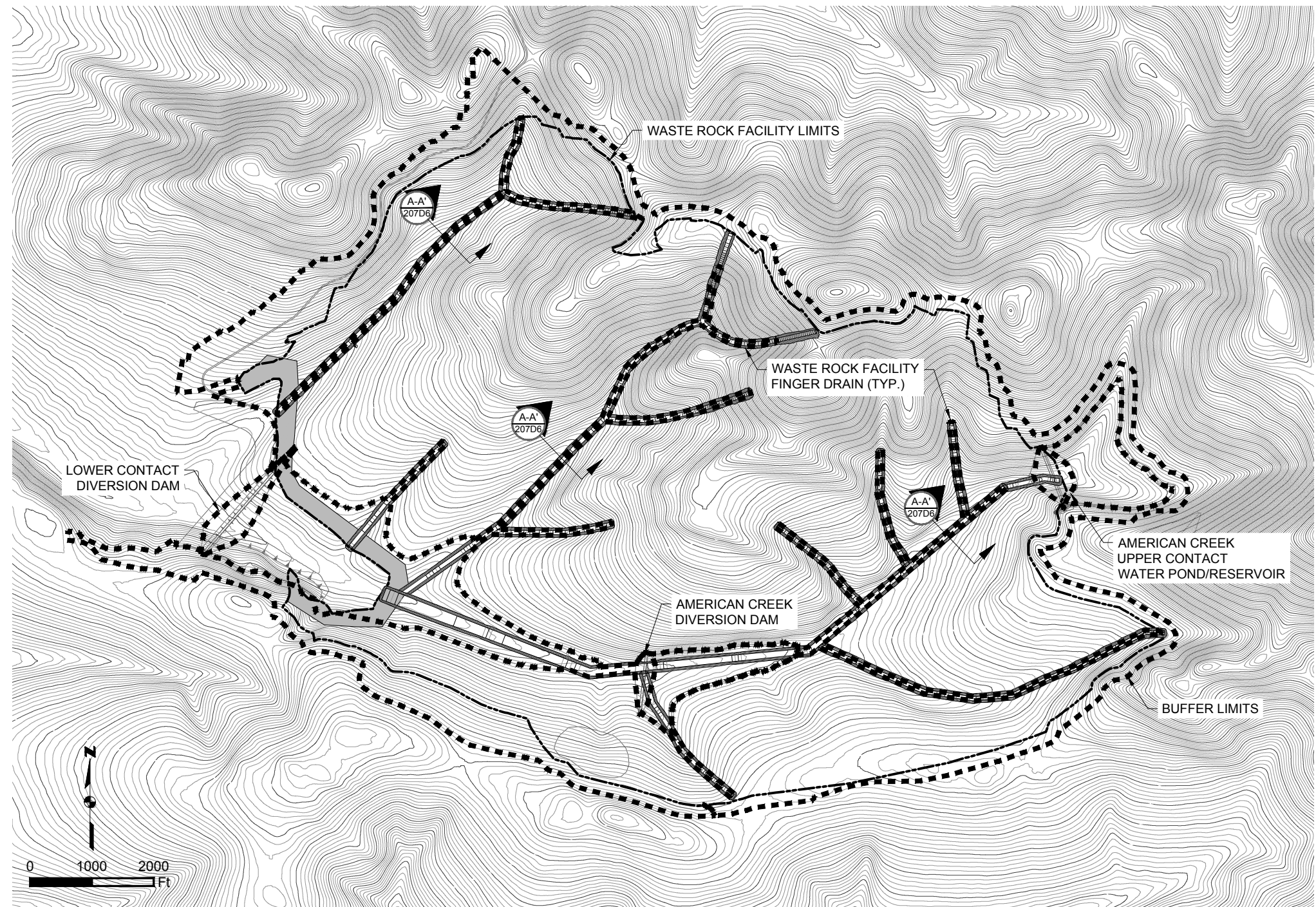
WASTE ROCK FACILITY DRAINAGE SYSTEM PLAN SCALE 1" = 2000'
