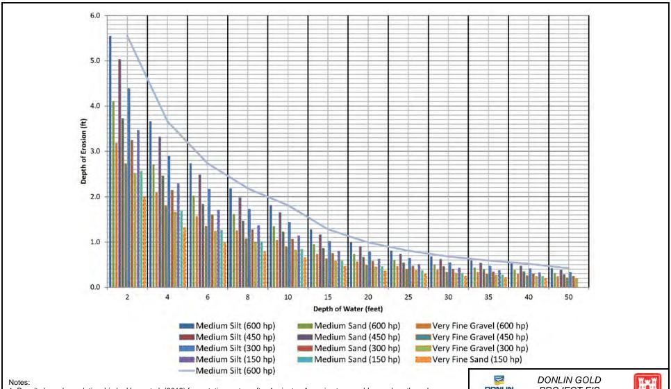
1. Results based on relationship by Hong et al. (2012) for a stationary tow after 1 minute. A moving tow would scour less than shown; e.g., a tow moving at 5 mph would move about 400 feet in 1 minute, so would likely scour less at any specific location within the 400-foot length.
