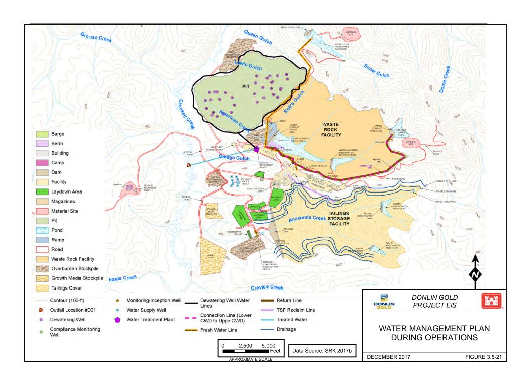
The Upper CWD would receive runoff from undisturbed ground above the dam and contact water pumped from the Lower CWD through an above ground pipeline. Transferring water from the Lower CWD to the Upper CWD would serve to minimize wetting of the toe (lower end) of the WRF. The pipeline route would follow the southern edge of the WRF (Figure 3.5-21).
