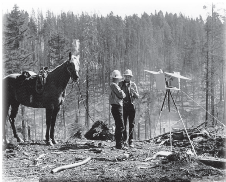
Using a portable weather station to gather fire weather data during the 1959 Brackett Creek Fire in the Gallatin National Forest (photo: USDA Forest Service).
