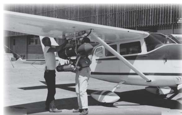
Mounting silver iodide generator for Project Skyfire, 1964 (photo: USDA Forest Service).
