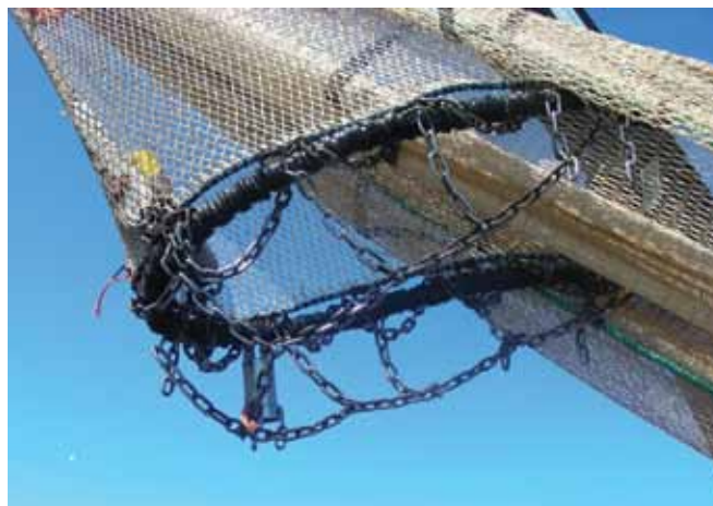
Photos from the 2007 BSFRF trawl showing footrope configuration along wing sections (left) and the throat section (right).
