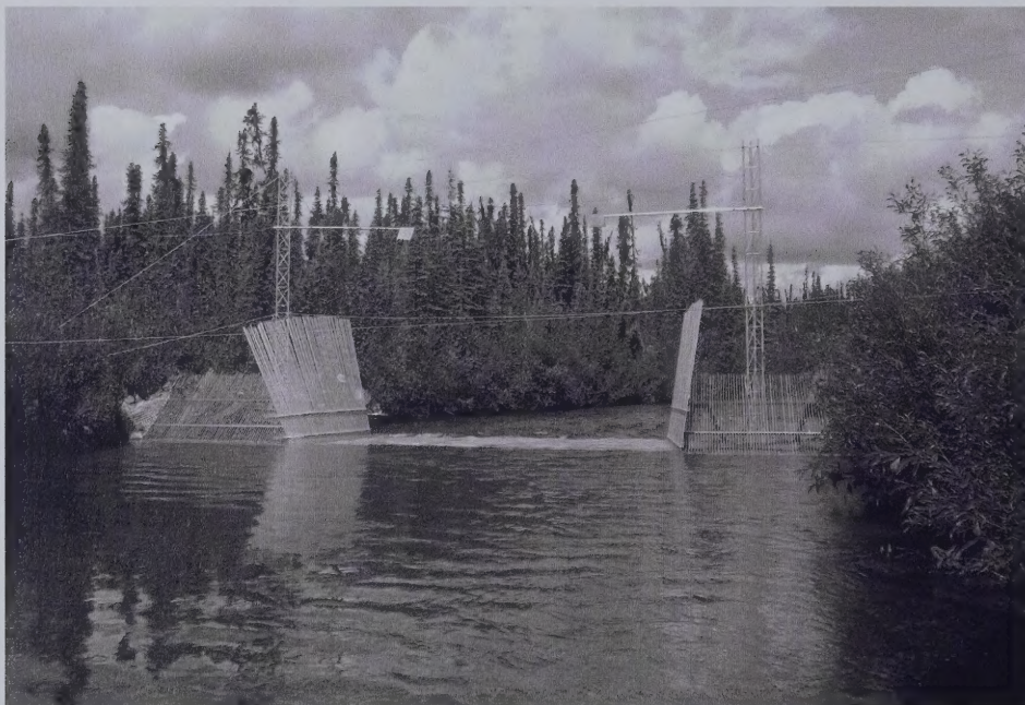
View of the project on Caribou Creek. Cameras are mounted on the horizontal arms hanging over the stream from the right and left.
