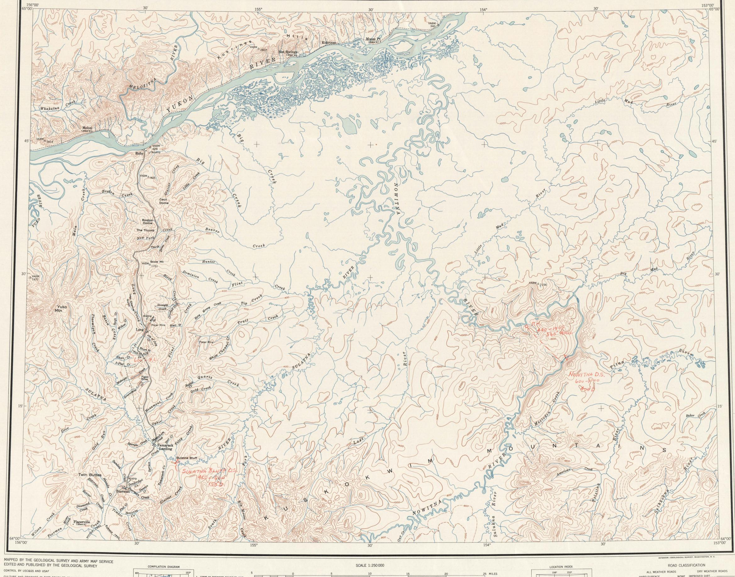
CONTROL BY USC&GS AND USAF CULTURE AND DRAINAGE IN PART COMPILED FROM TRIMETROGON PHOTOGRAPHY. TOPOGRAPHY COMPILED FROM ORIGINAL SURVEYS OF THE GEOLOGICAL SURVEY AND OTHER OFFICIAL SOURCES 1909-1915. SUPPLEMENTED BY STEREOPHOTOGRAMMETRIC (PHOTOALIDADE AND MULTIPLEX) COMPILATION, 1943-1945 UNIVERSAL TRANSVERSE MERCATOR PROJECTION, ZONE 5
