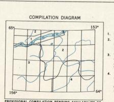
CORPS OF ENGINEERS MULTIPLEX, 1945 TOPOGRAPHY BY PHOTOALIDADE METHODS 1945, TRANSFERRED AND ADJUSTED TO TRIMETROGON BASE
