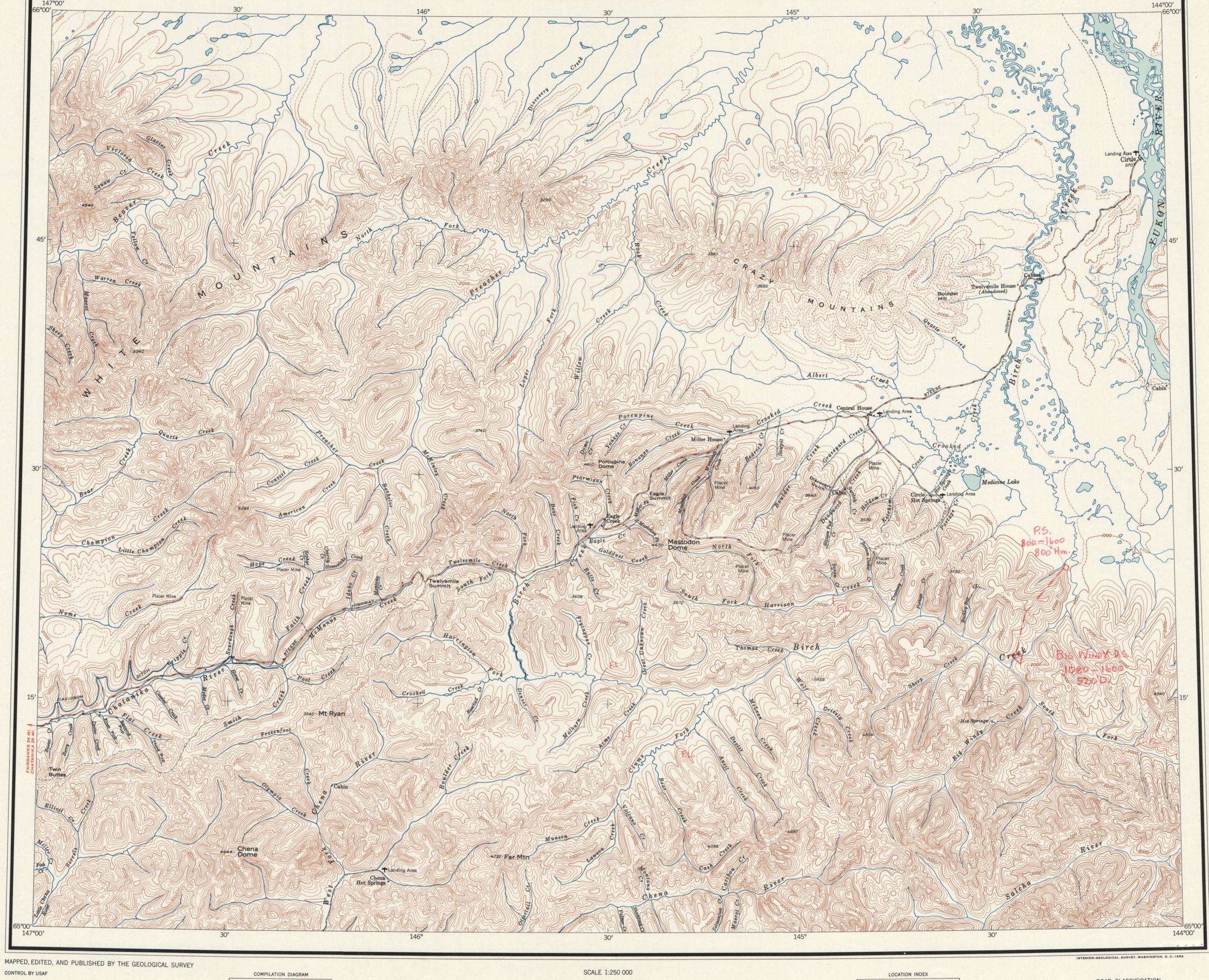
CULTURE AND DRAINAGE IN PART COMPILED FROM TRIMETROGON PHOTOGRAPHY, 1941-1947. TOPOGRAPHY COMPILED FROM ORIGINAL SURVEYS OF THE GEOLOGICAL SURVEY AND OTHER OFFICIAL SOURCES 1903-1908, SUPPLEMENTED BY STEREOPHOTOGRAMMETRIC (PHOTOALIDADE AND MULTIPLEX) COMPILATION, 1945
