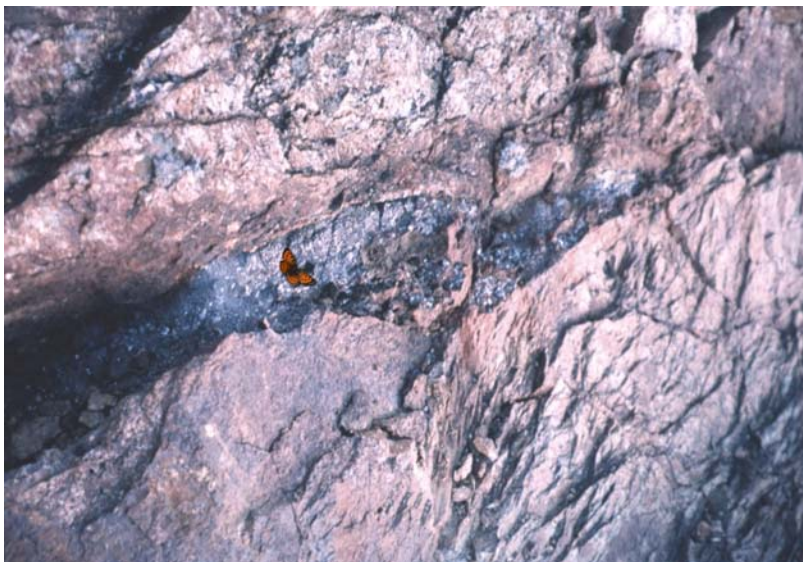
Photo 25. Silver-rich galena vein in the east shear of the North Marsha Peak prospect. Note butterfly for scale. Photo by J. Still.
