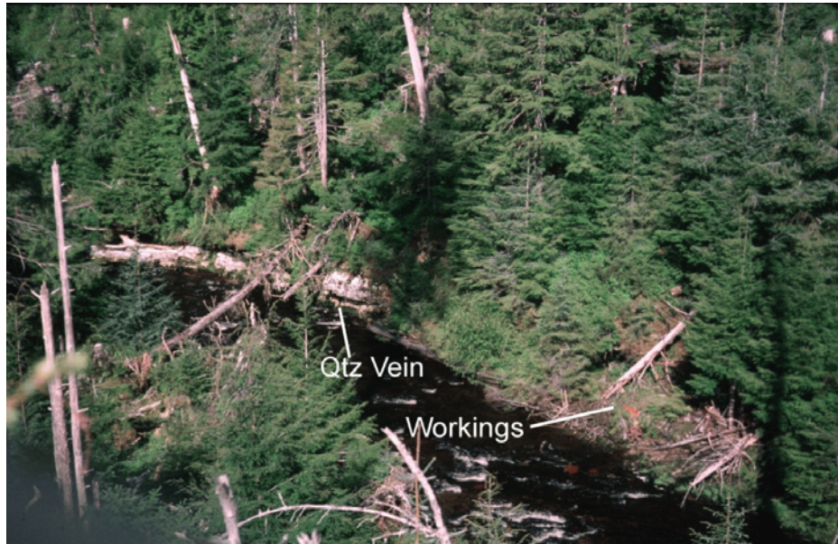
Photo 18. A thick quartz vein and remains of workings at the K & D Mine. Current access to the adit is through a makeshift portal under the large fallen tree near the workings. Photo by K. Bean.
