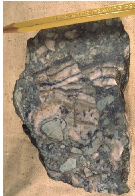
Photo 5. Mineralized breccia of green tuff. Seams and disseminations of galena and sphalerite with pink barite. Photo by P. Bittenbender.
