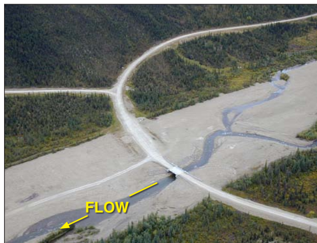
Figure 9. Aerial view of the channel upstream of the bridge, where the gabions are being eroded by the unstable channel.
