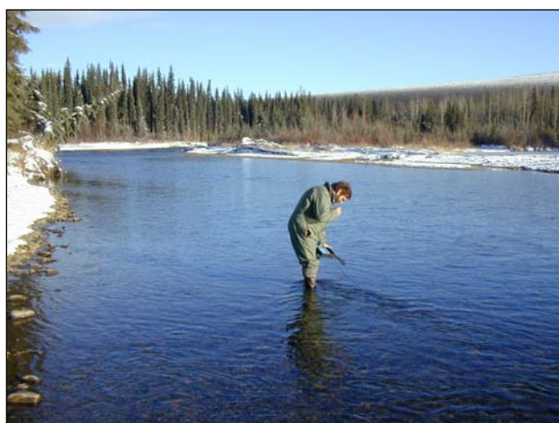
Figure 6. Water-quality readings were taken in-situ with single parameter meters.
