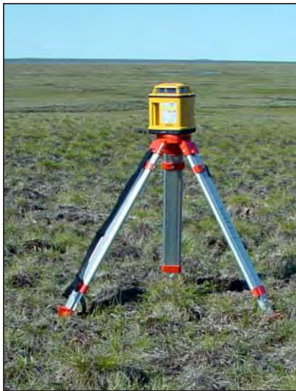
Figure 12. Depth to permafrost measurements using the Laser Alignment LB-9 Laser Beacon.
