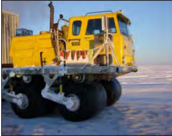
Figure 5. Balloon tires on rolligon trucks provide low impact.
