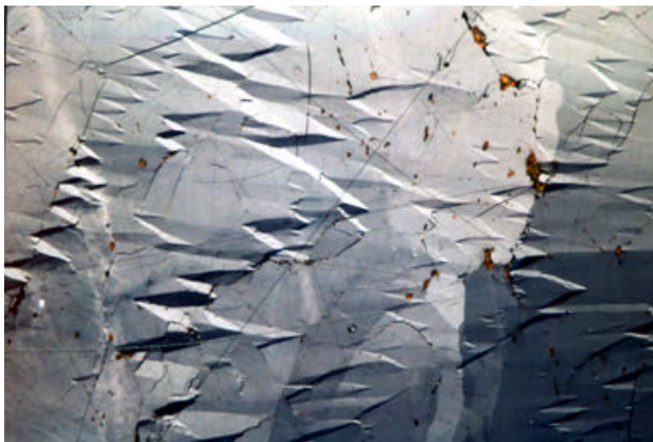
Fig.26: Photomicrograph of euhedral stibnite (antimonite) mineralization. Reflected light on polished surface, oil immersion, crossed-polars. Bottom edge of picture is 0.7 mm in length.
