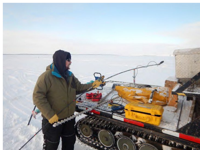
Photo 3.4: Attaching Hach flow meter to fixed rod at Ocean Point Upstream; 2/25/20
