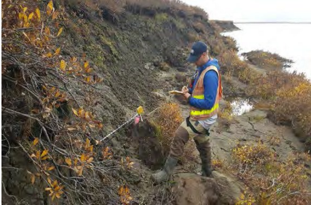
Photo 3.3: Investigating soil active layer at Ocean Point Downstream Transect; right/east bank; 9/14/19
