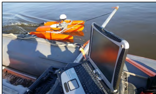
Photo 1. Discharge measurement in progress at Transect #1; Sept 5, 2019
