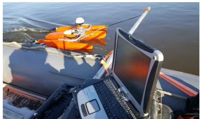
Photo 3.1: Discharge measurement at Ocean Point Upstream Transect; 9/5/19
