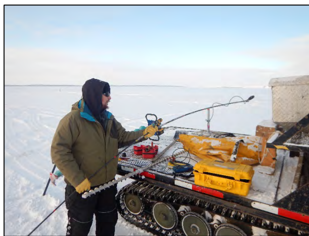
Photo 3.4: Attaching Hach flow meter to fixed rod at Ocean Point Upstream; 2/25/20
