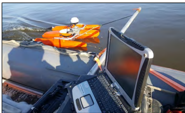
Photo 3.1: Discharge measurement at Ocean Point Upstream Transect; 9/5/19
