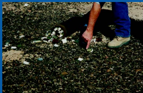
Figure 30 – A 155 mm artillery dispenser carries grenade-like submunitions to the target. This dispenser did not open properly to scatter the submunitions; the inert submunitions fell out when the round hit the ground. Submunitions are small and often do not look like military munitions.
