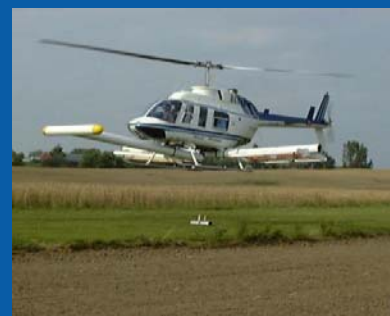
Figure 15 – Helicopter configured with magnetometers for UXO and DMM detection. Photo courtesy of Oak Ridge National Laboratory.
