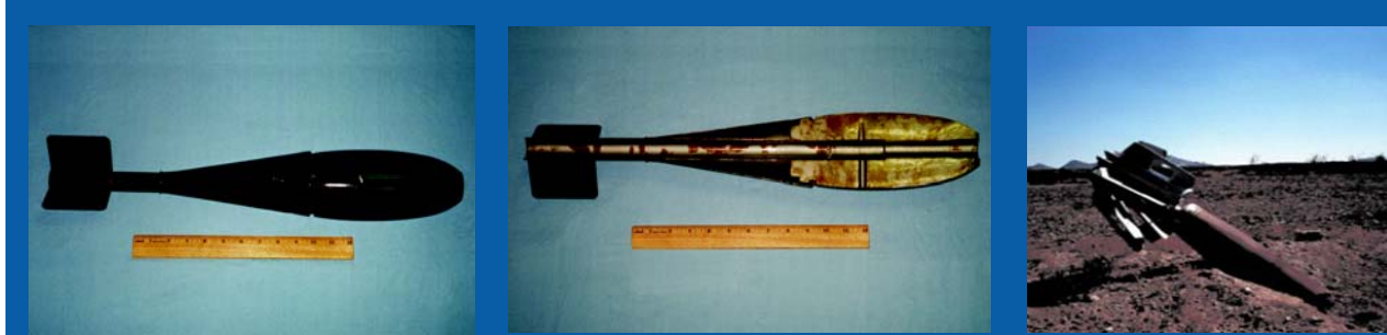
Figure 29 –Left and center: Practice bomb (BDU-33) and a cutaway of the bomb. This practice bomb is approximately 2 feet long. The central channel in the bomb contains an explosive spotting charge large enough to cause serious injury. (Note: Practice munitions are painted blue, but not all blue munitions are necessarily inert.) Right: Bomb found on public lands north of Chocolate Mountains Gunnery Range, California.
