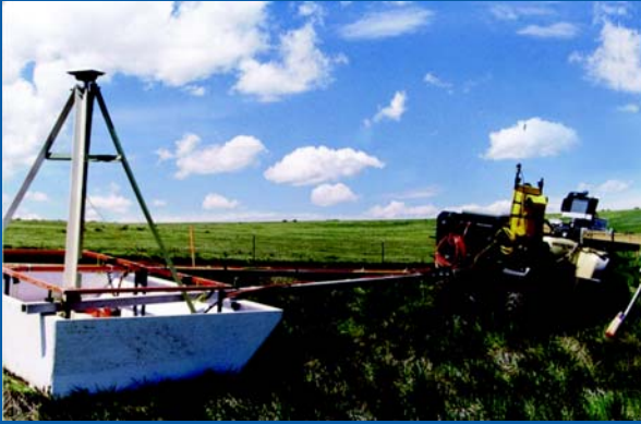
Figure 22 – Ground penetrating radar sled in towed configuration. Photo courtesy of Blackhawk Geometrics.
