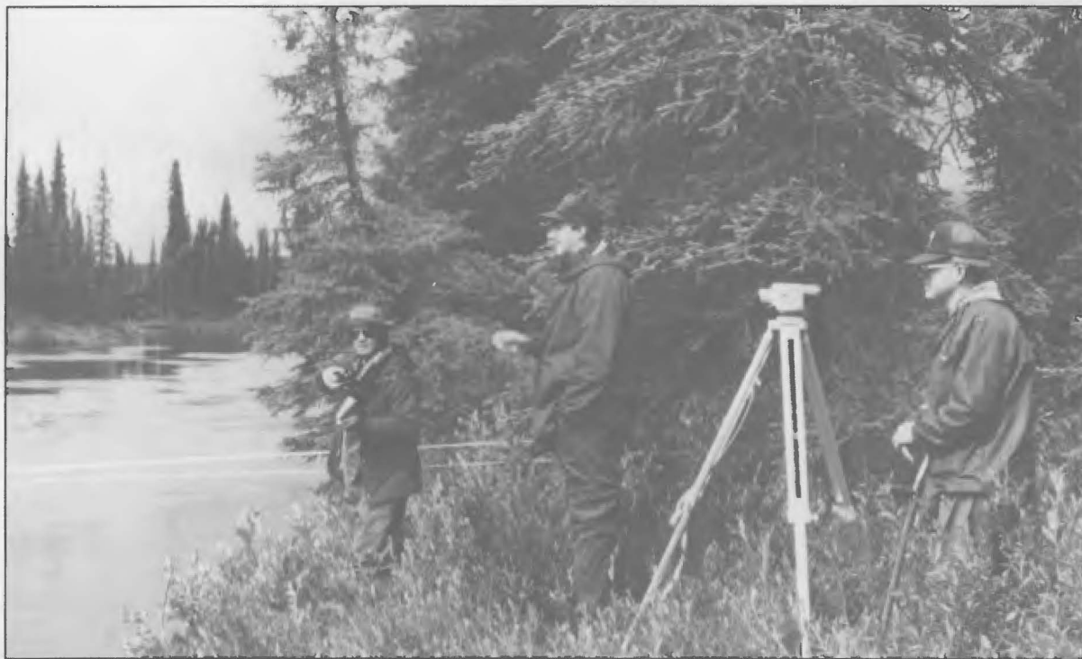
Figure 6. Hydraulic geometry data were developed from surveys of 31 channel cross-section sites on the Gulkana National Wild River.
