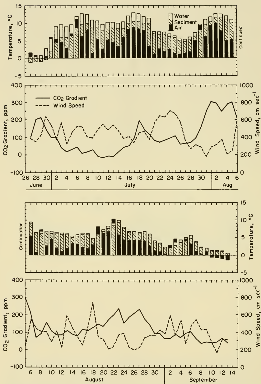
FIGURE 4-10. Mean daily air, water, and sediment temperatures, mean wind speed, and mean gradient of p\text{CO}_2 (water minus air) in North Meadow Lake, 1972. (After Coyne and Kelley, 1974.)
