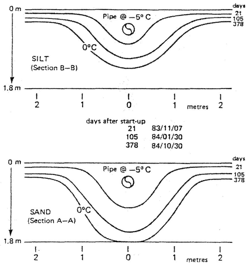
Figure 4.1: Sections showing evolution of frost bulb around pipeline in sand and silt.
