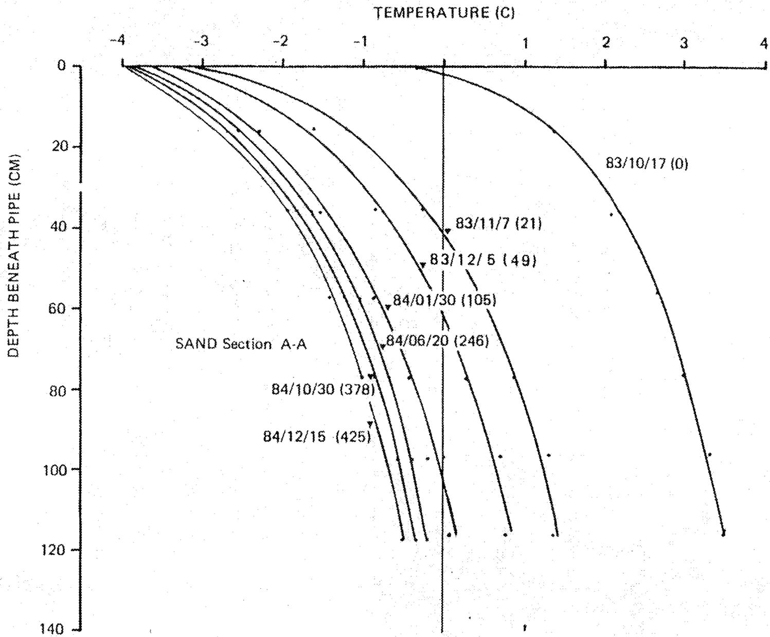
penetration beneath the bottom of the pit under the centre line of the pipeline. The average thermal gradient in the frozen portion of the sand was about 2.6 °C/m.
