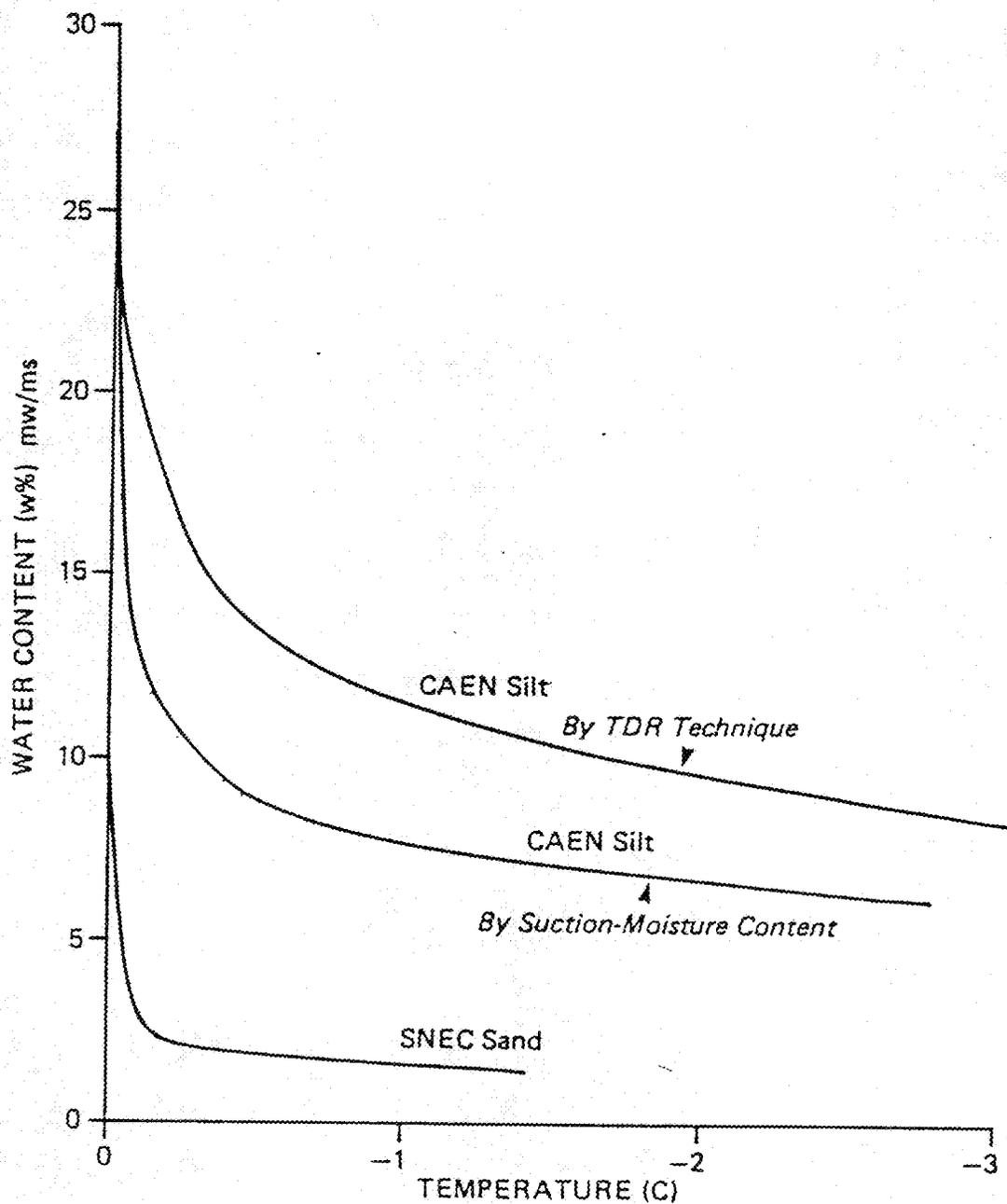
Figure 3.7: Unfrozen water content vs temperature for Caen silt and SNEC sand
