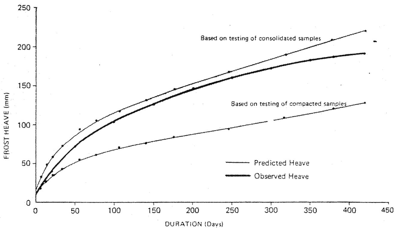
Figure 6.1: Predicted and observed heave for Caen experiment (silt section B-B)
