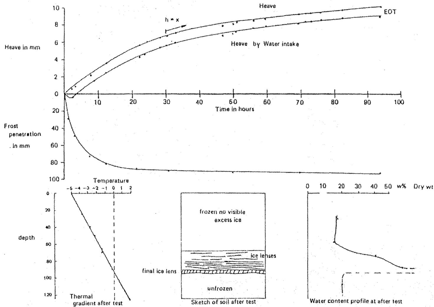
Figure 5.4: Typical results from frost heave test on Caen silt (test results shown for test SRD 9)
