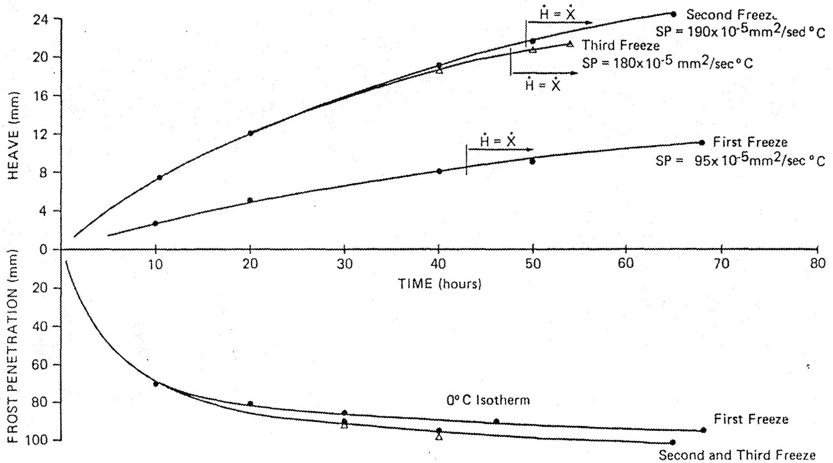
Notes: Results from Exp. SRD 10a, b, c  $T_c = -3.0^\circ\text{C}$ ,  $T_w = +1^\circ\text{C}$ ,  $\rho_d = 1.73 \times 10^3 \text{ Kg/m}^3$
