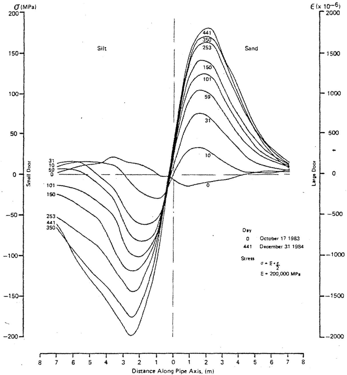
Figure 4.9: Distribution of axial bending stress and pipe strain during second freeze period.
