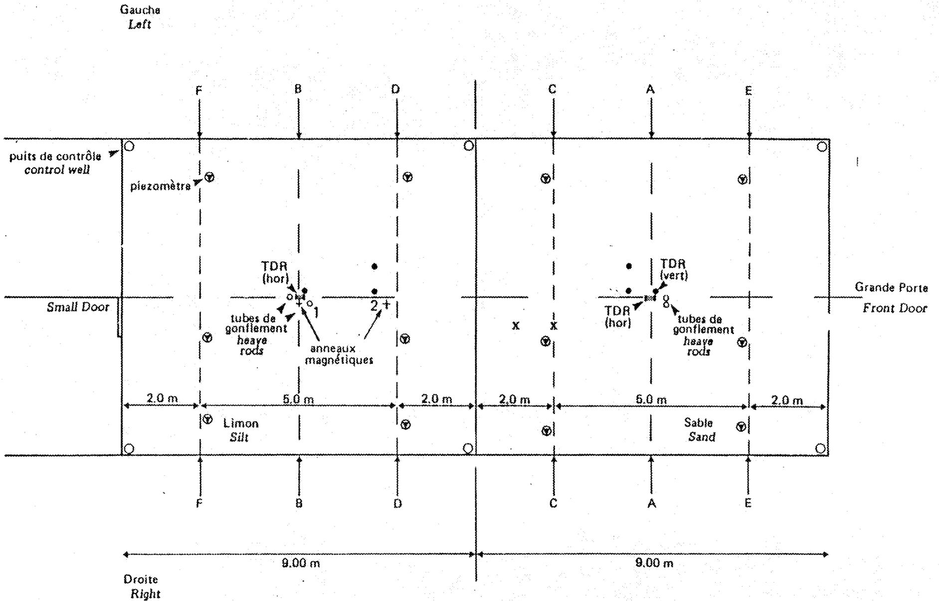
Figure 3.3: Plan view of Caen experiment showing location of surface instrumentation and instrumented sections.
