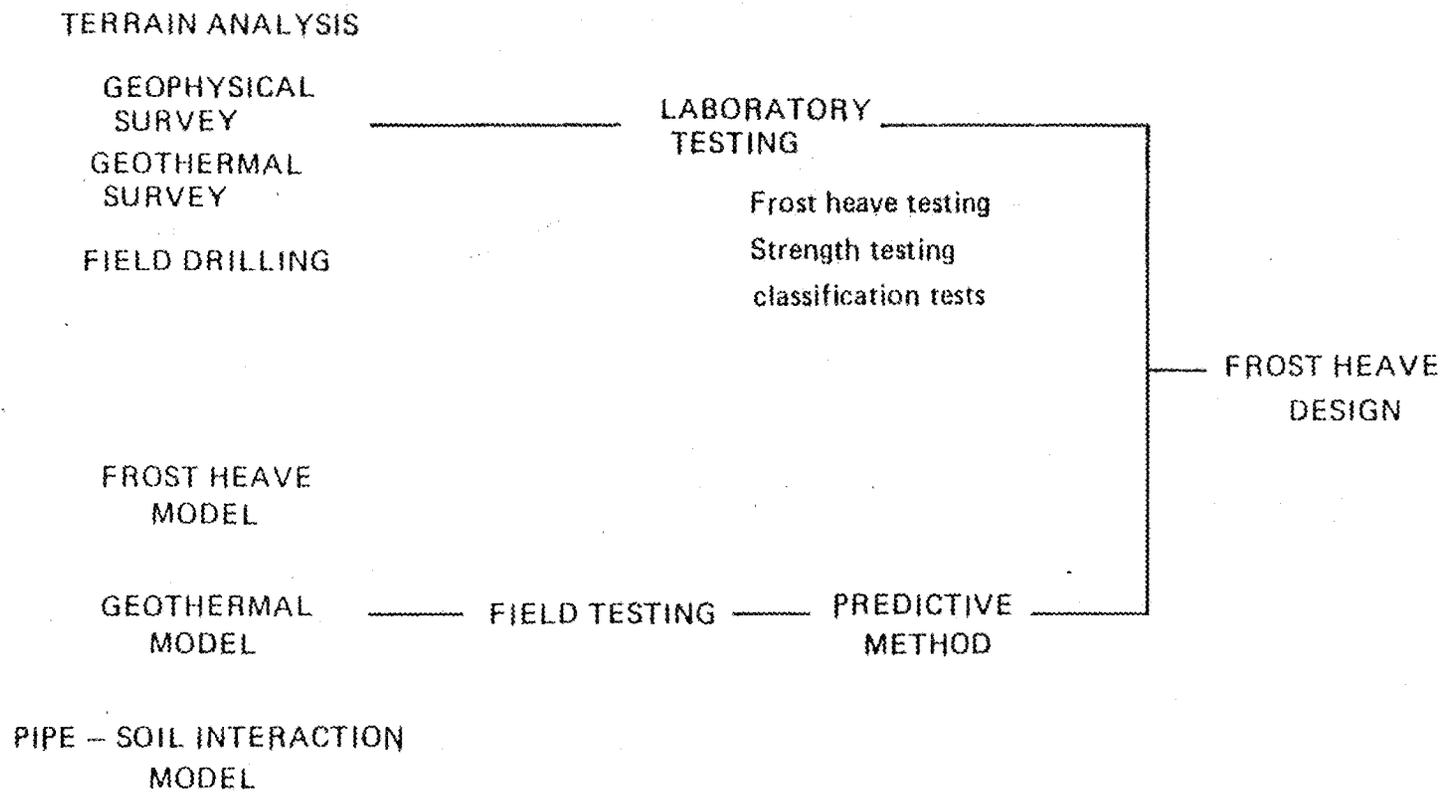
Figure 2.3: FROST HEAVE DESIGN PROGRAM FOR A CHILLED PIPELINE
