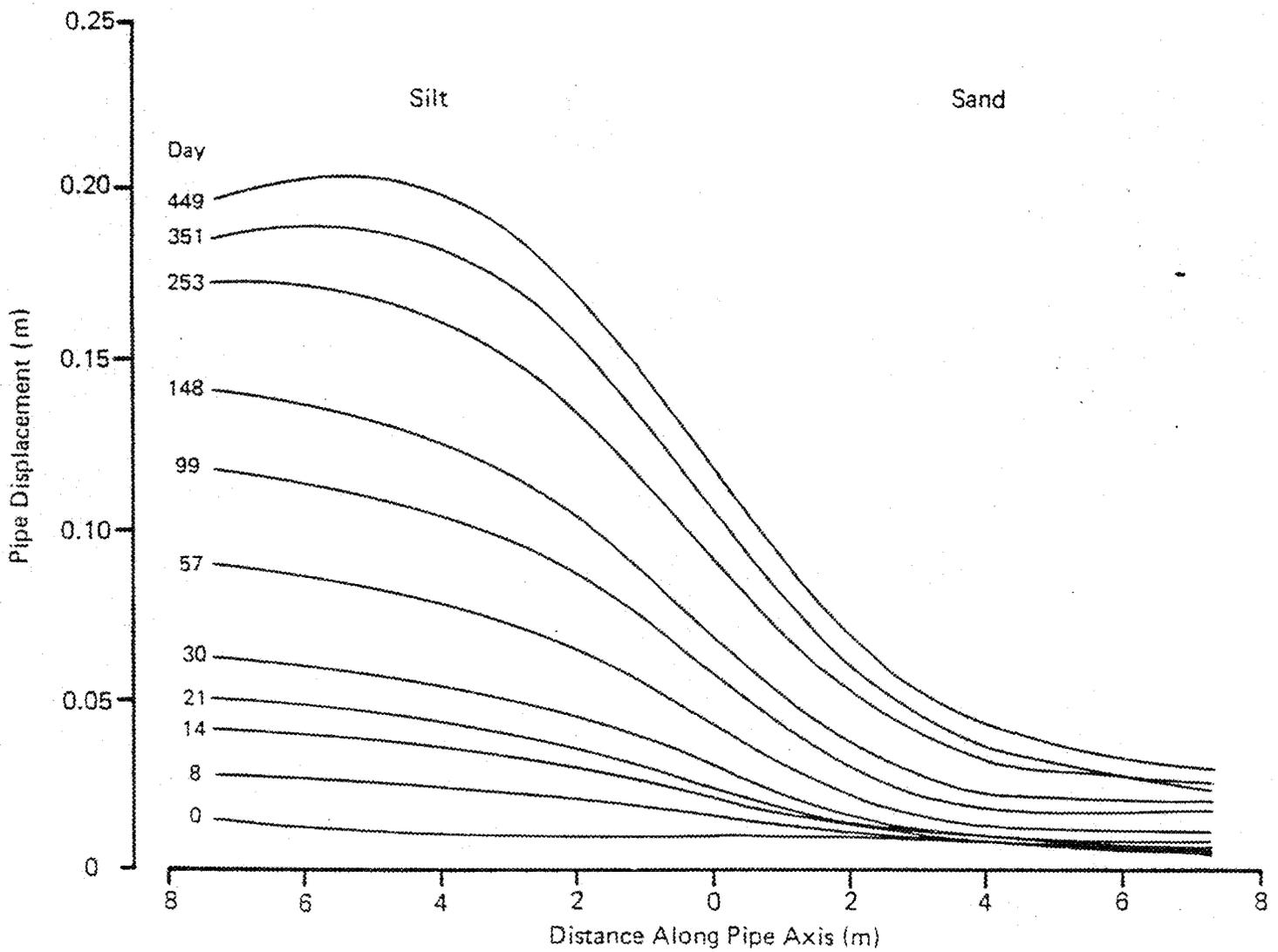
Figure 4.8: Displacement of Caen pipeline during second freeze period.
