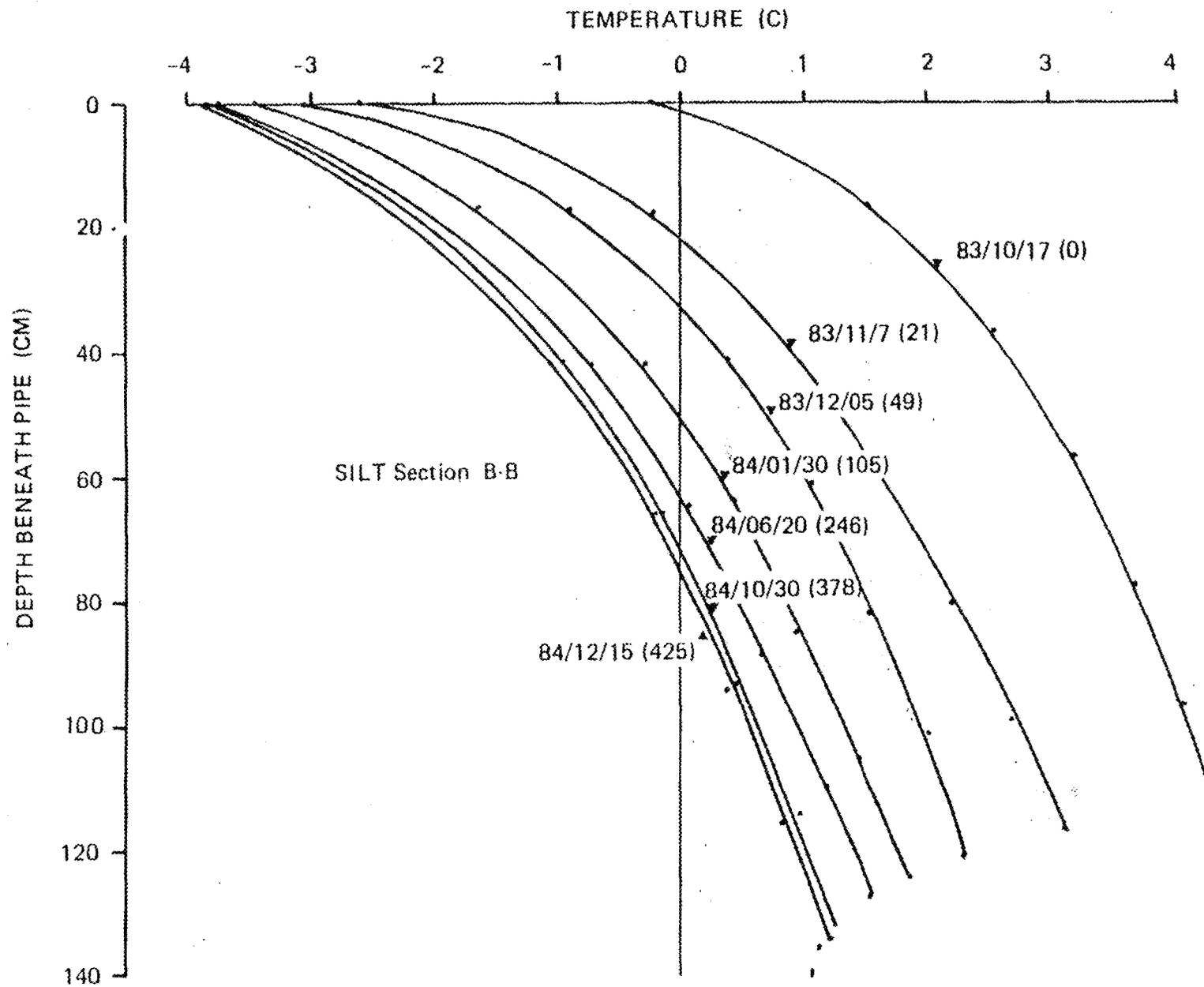
Figure 4.2: Temperature profiles beneath pipe in silt
