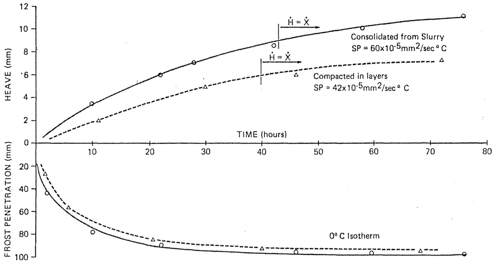
Notes: Results from Exp. SRD 6,9  $T_c = -5.0^\circ \text{C}$ ,  $T_w = +1.5^\circ \text{C}$ ,  $\rho_d = 1.73 \times 10^3 \text{ Kg/m}^3$
