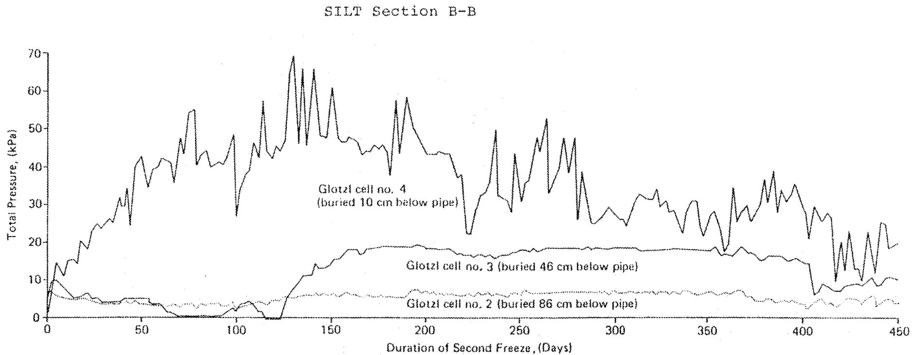
Figure 4.12: Total stress measured in soil beneath the centre line of the pipeline in the silt
