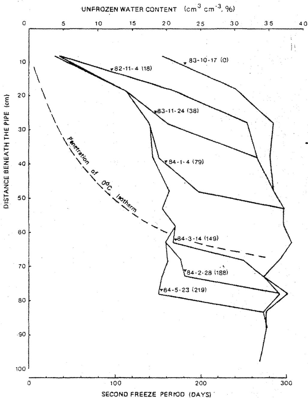
Figure 4.4: Unfrozen water content profiles and progression of  $0^\circ\text{C}$  isotherm beneath pipe in silt (section B-B).
