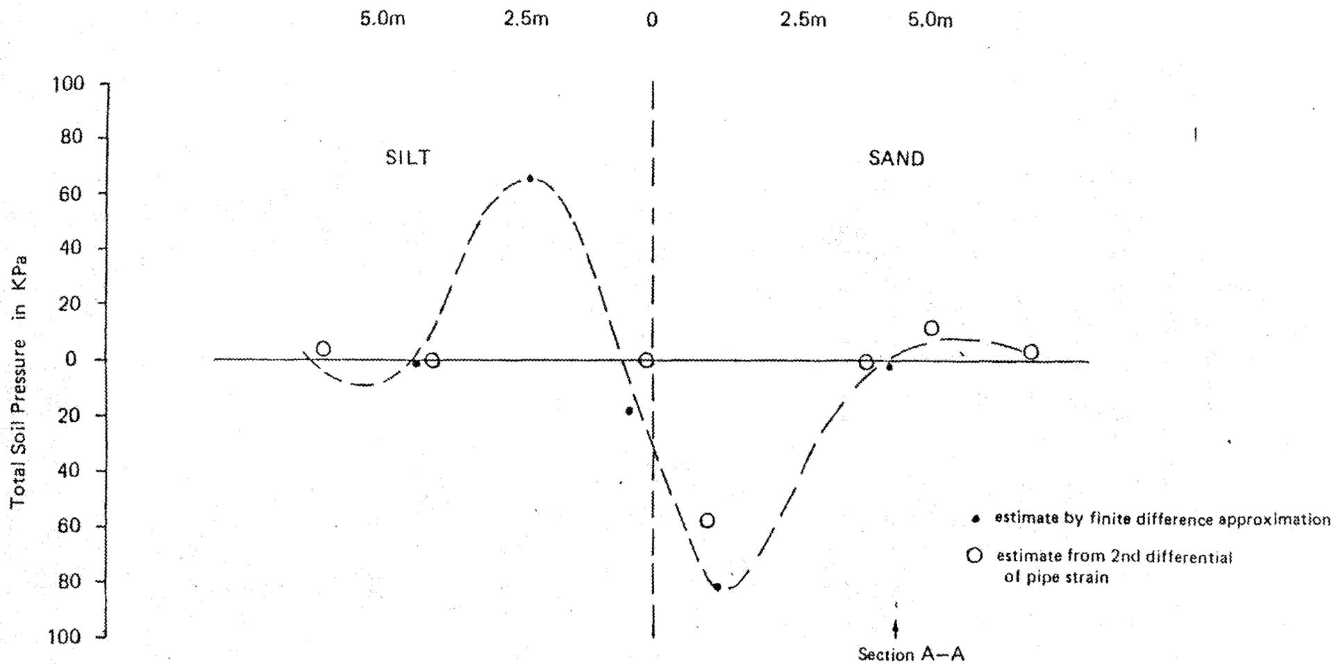
Figure 4.10: Estimate of soil pressure beneath pipe as determined from pipe stress measurements.
