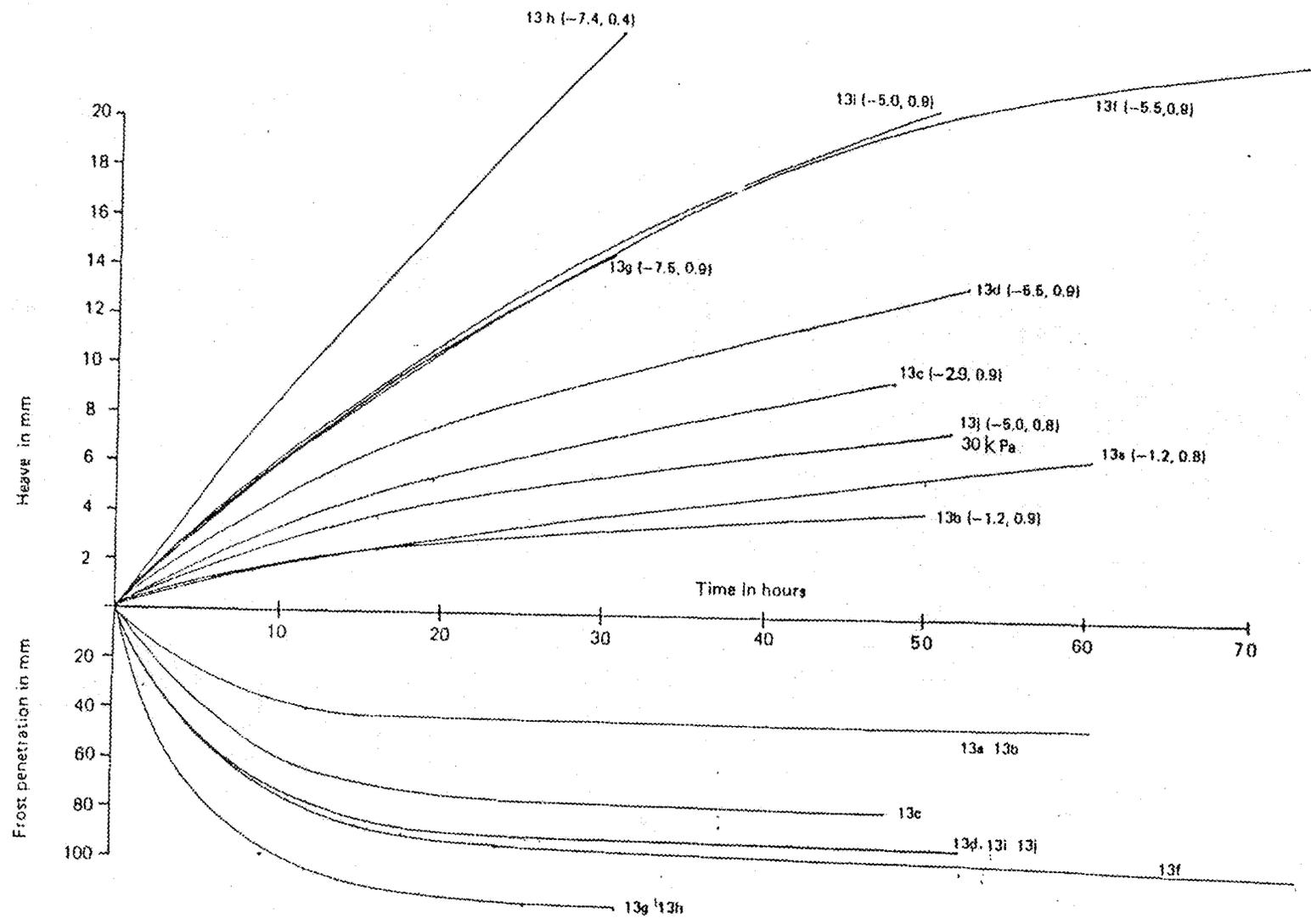
Figure 5.7: Influence of repetitive freeze-thaw cycles under different temperature conditions.
