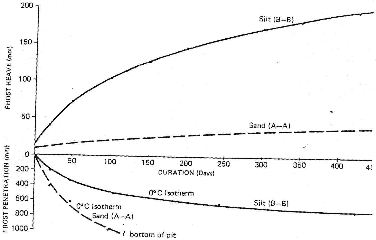
Figure 4.6: Frost heave and frost penetration beneath the Caen pipeline.
