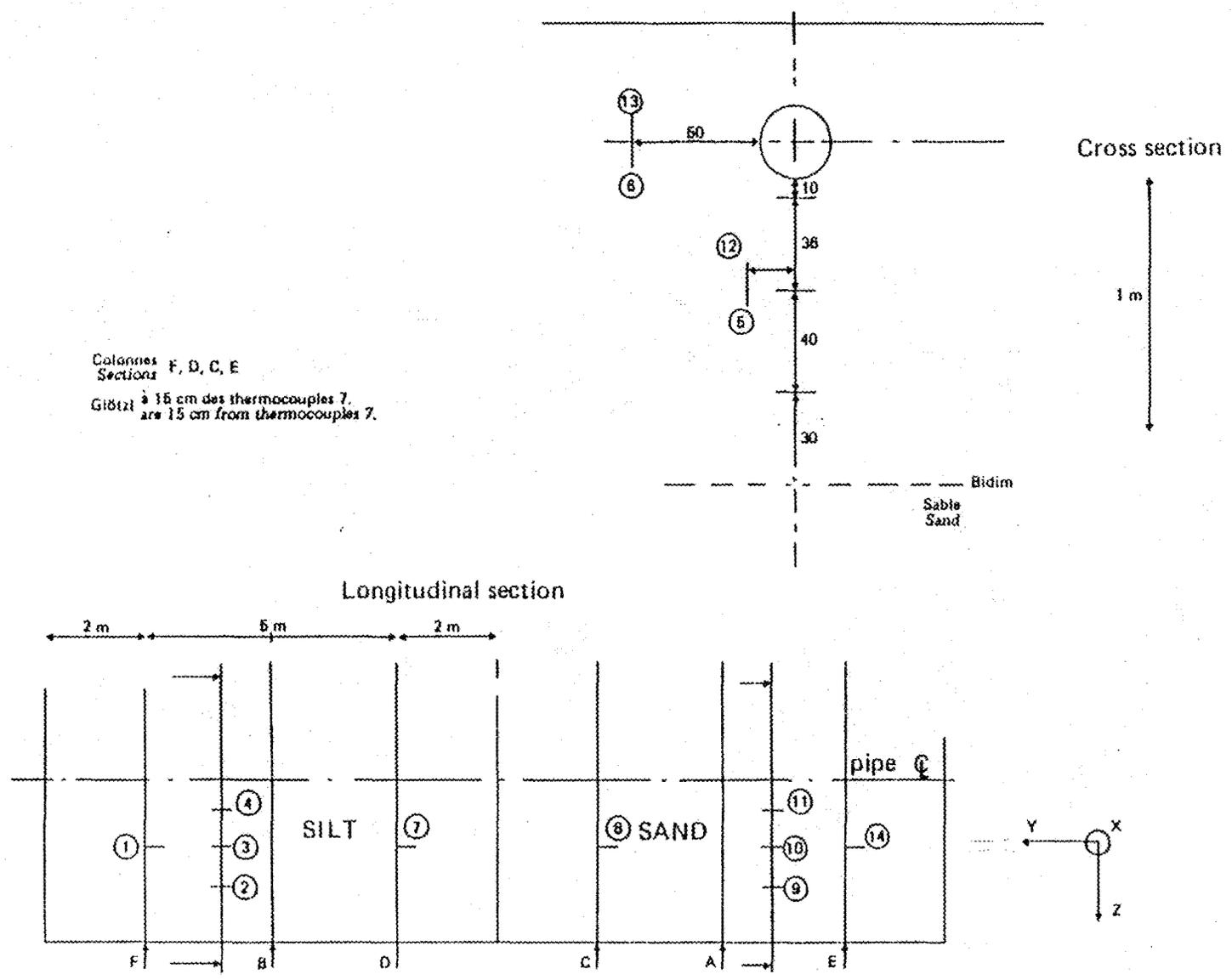
Figure 3.5: Location of earth pressure (Glötzl) cells
