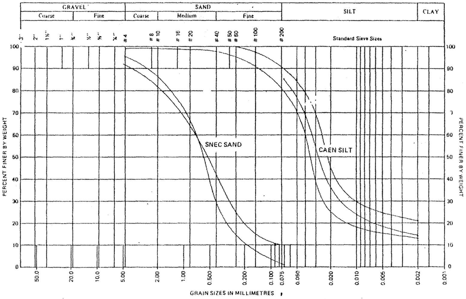
Figure 3.6: Grain size analyses of Caen silt and SNEC sand
