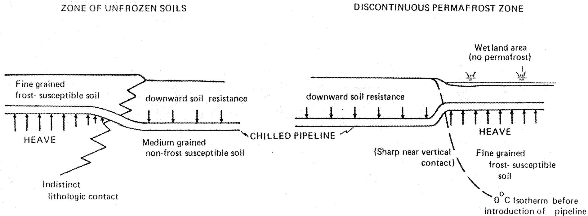
Figure 2.2: Differential frost heave occurring around a chilled pipeline. Case a) heave over indistinct lithologic contact, Case b) heave over sharp near vertical contact between frozen and unfrozen soil.
