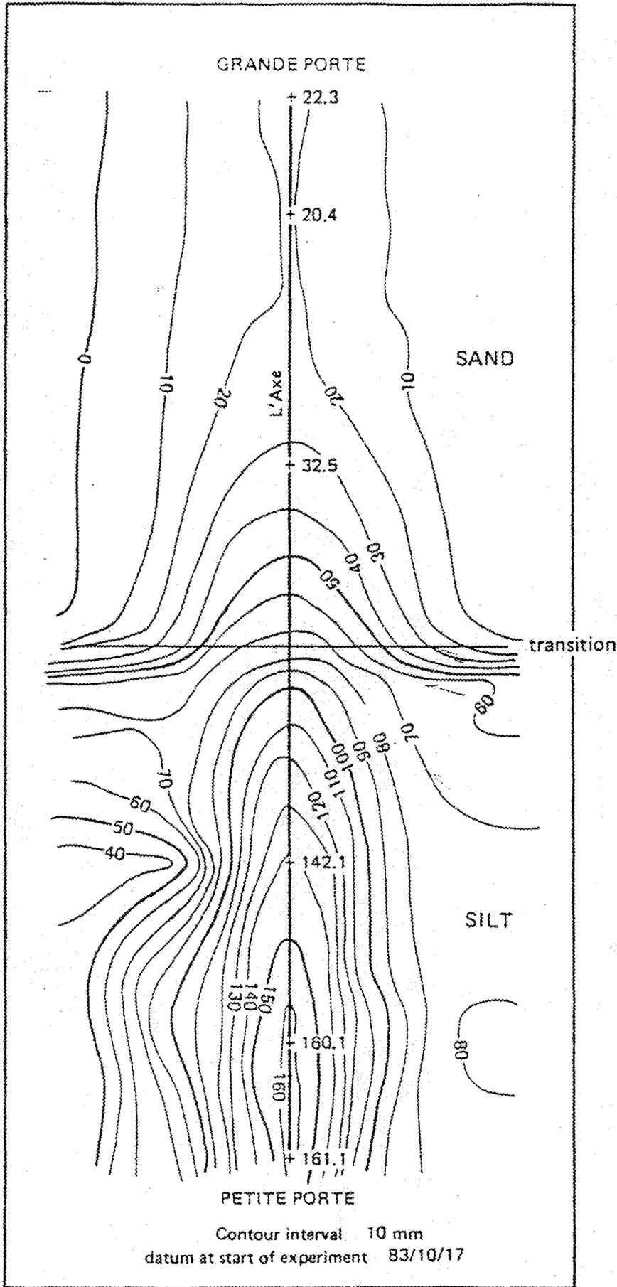
Figure 4.5 Change in surface elevations after 227 days of freezing
