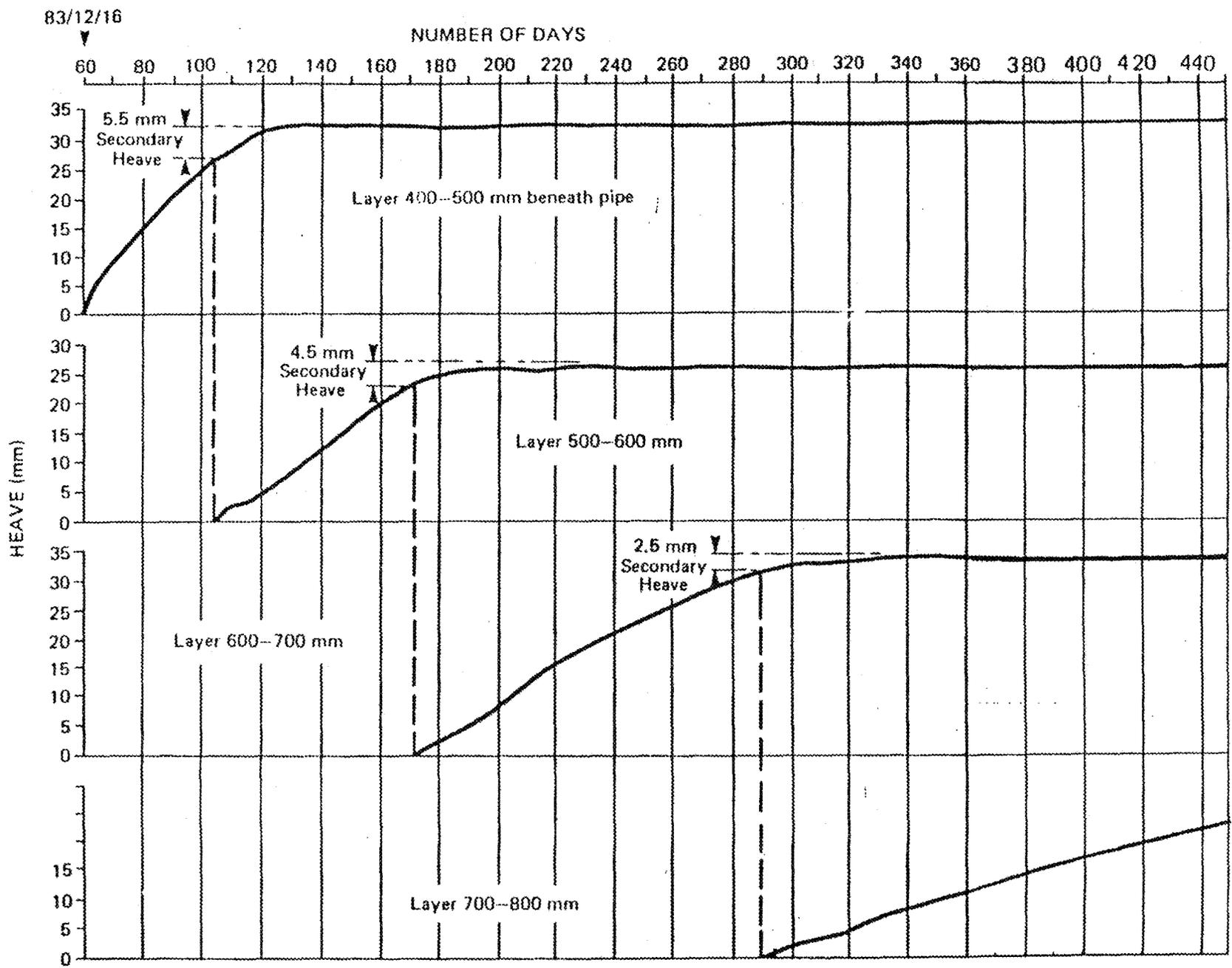
Figure 4.7: Differential heave with depth as determined with telescopic tubes
