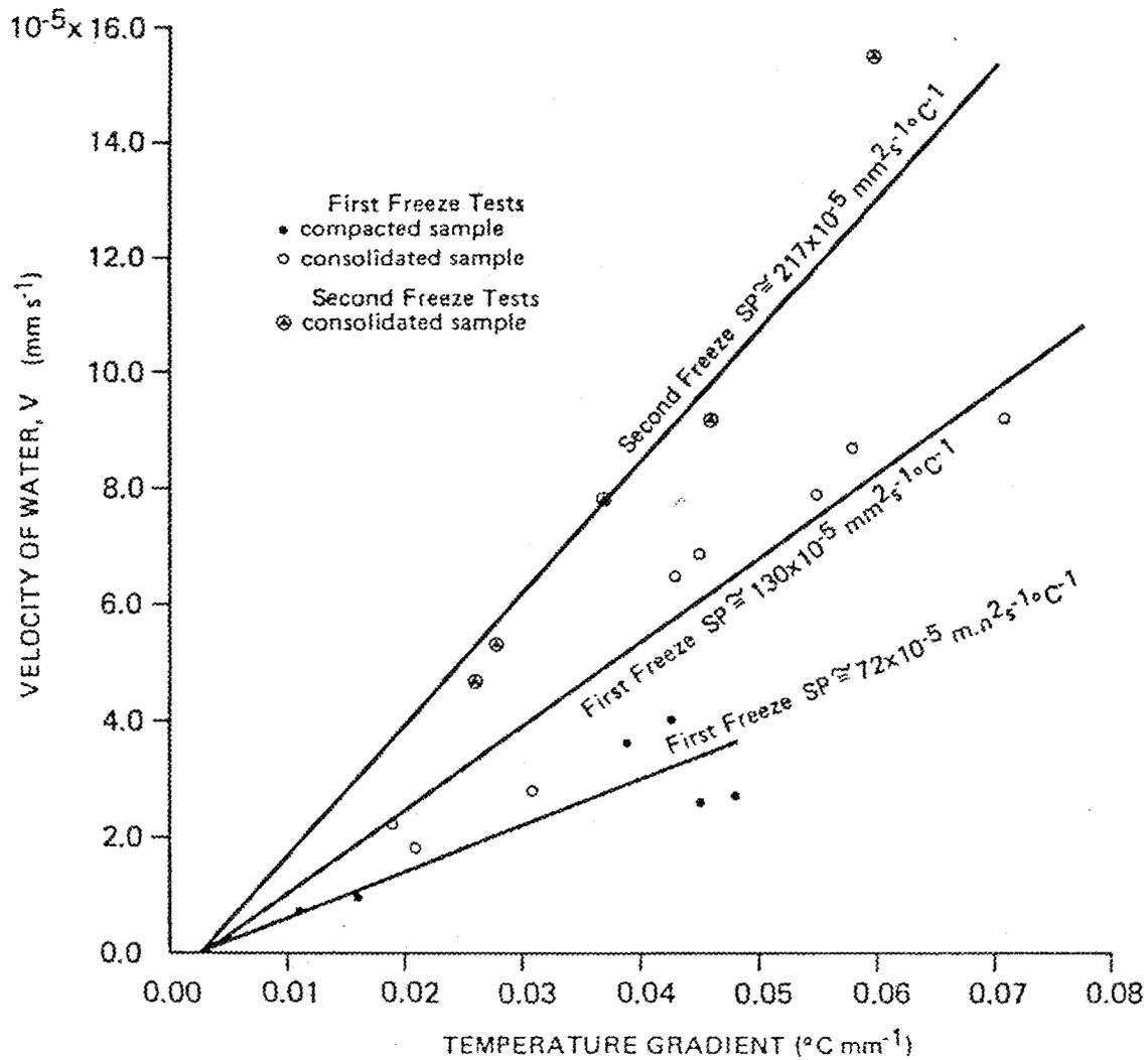
Figure 5.10: Plot of velocity of water flowing towards final ice lens vs temperature gradient of frozen fringe.
