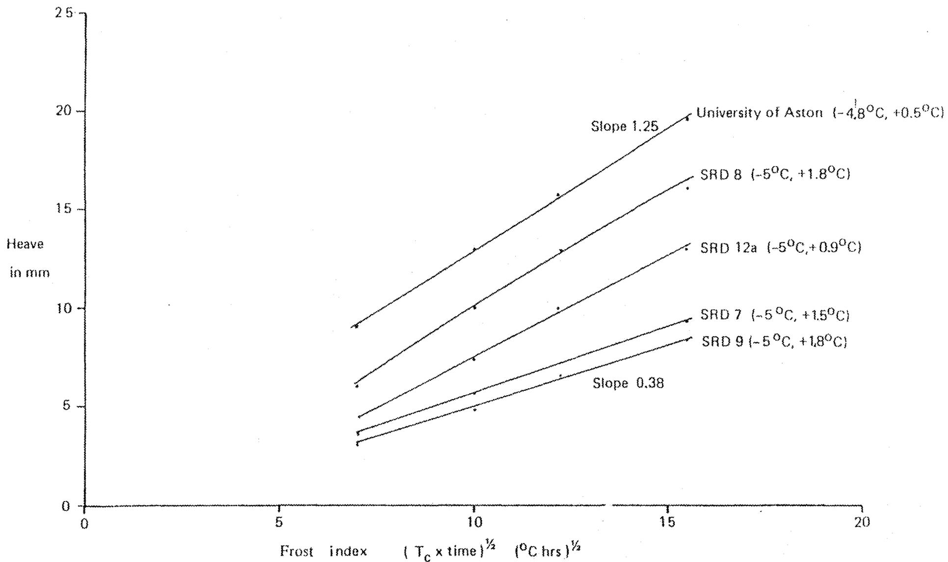
Figure 5.9 : Heave of Caen silt vs Frost index
