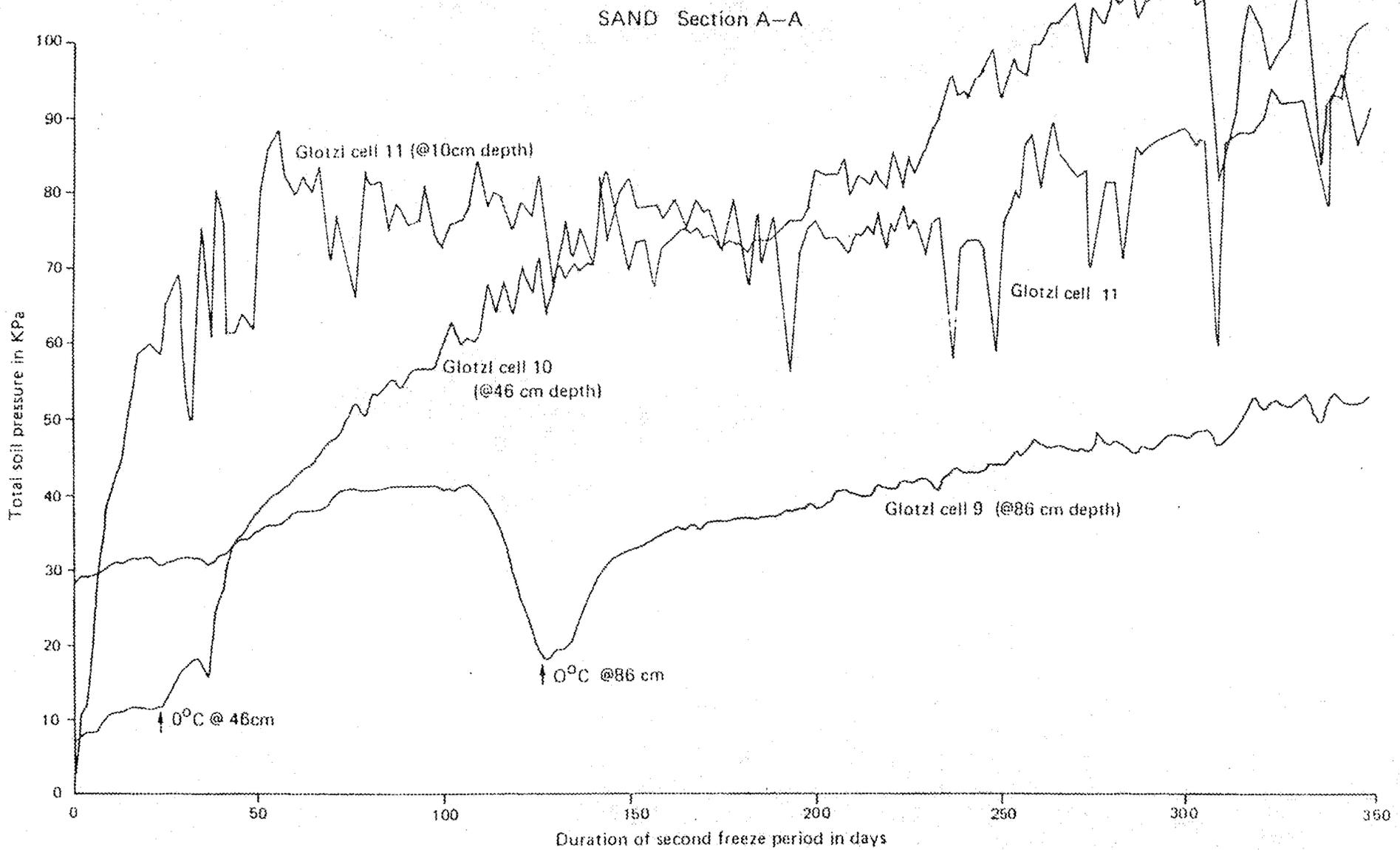
Figure 4.11: Total stress measured in soil beneath the centre line of pipe in sand.
