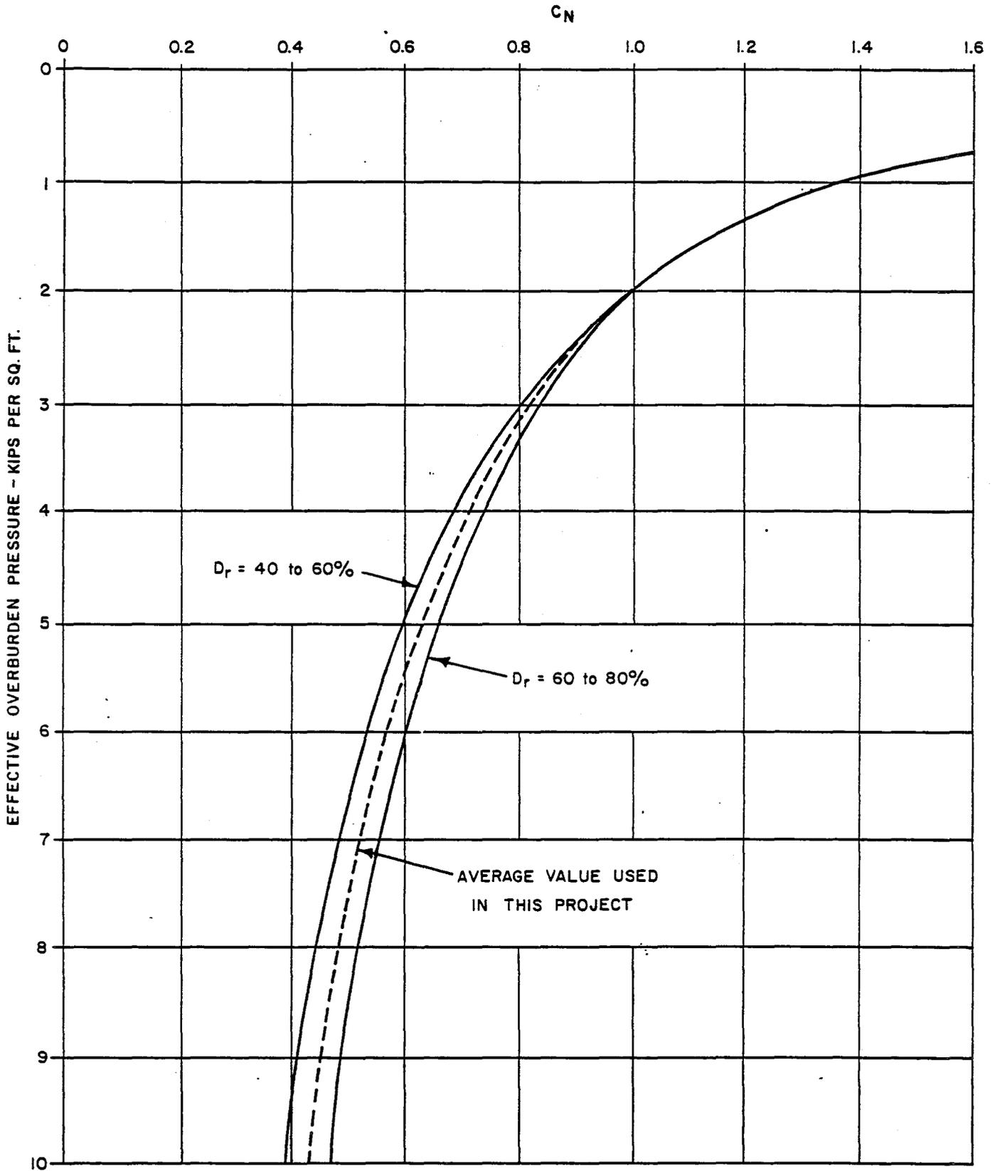
FIG. 5-62 Recommended Curves for Determination of  $C_N$  Based on Averages for W.E.S. Tests
