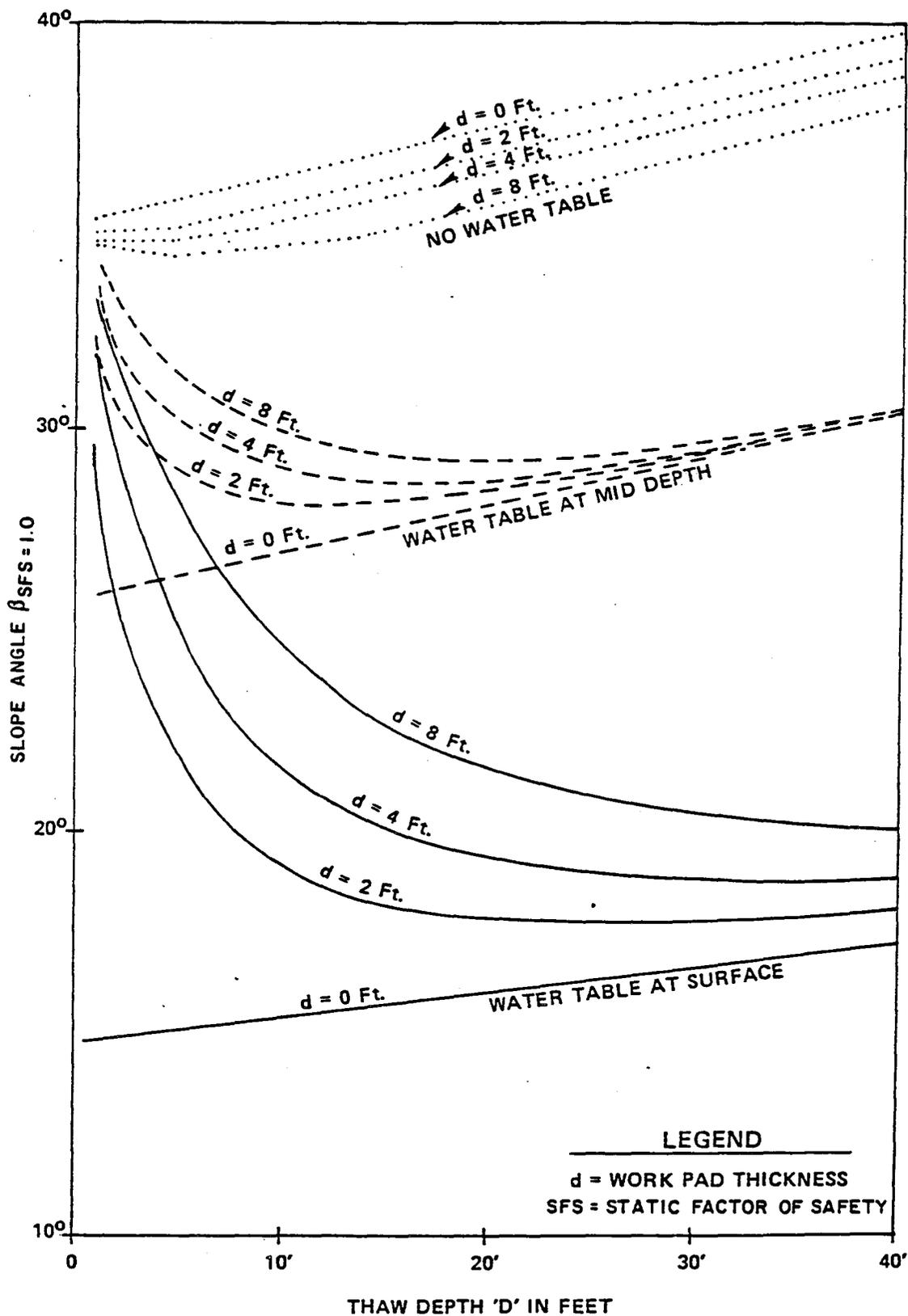
FIG. 5-17 SLOPE ANGLE FOR SFS = 1.0 vs. THAW DEPTH
