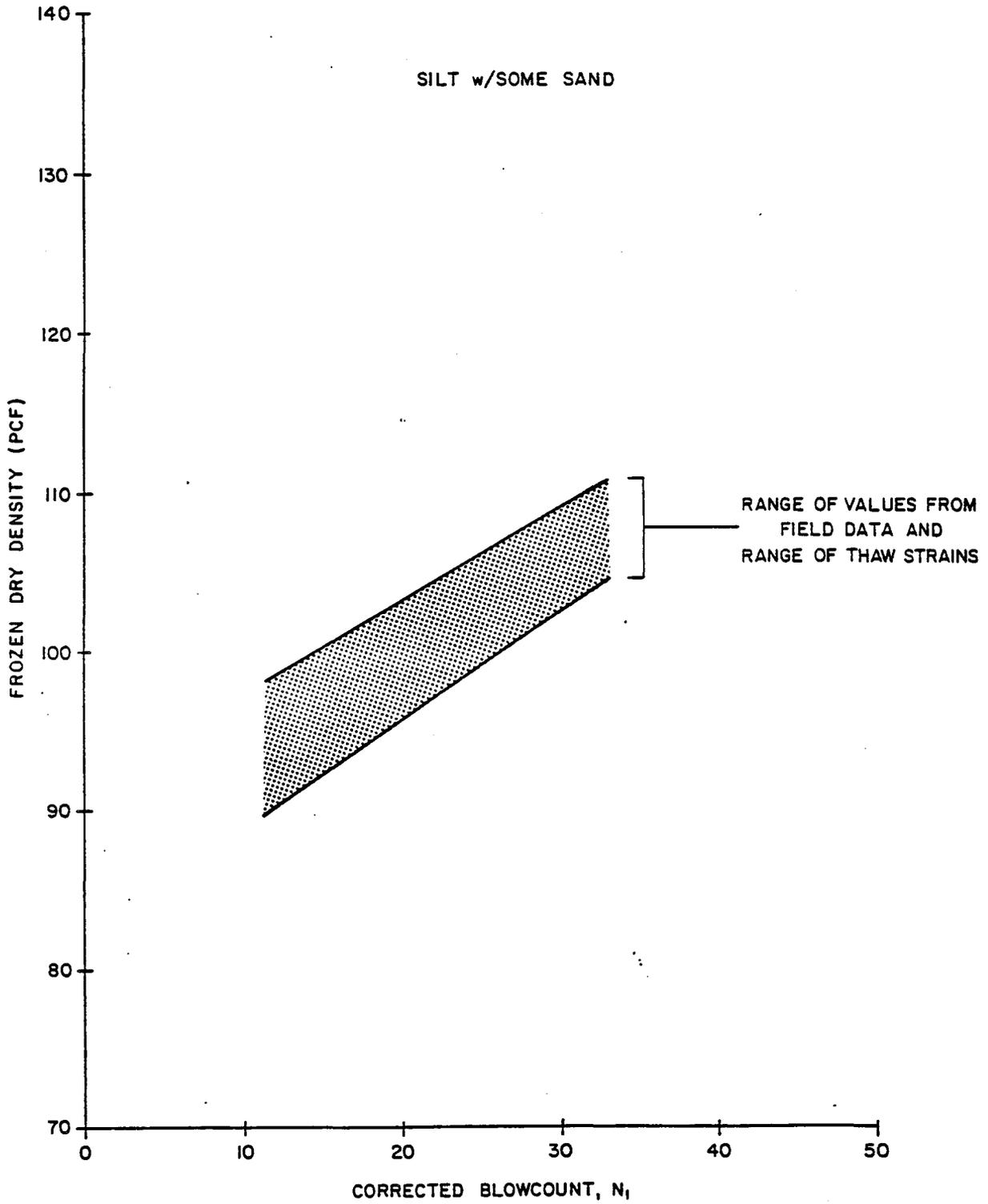
FIG. 5-63 FROZEN DRY DENSITY VERSUS CORRECTED BLOW COUNT
