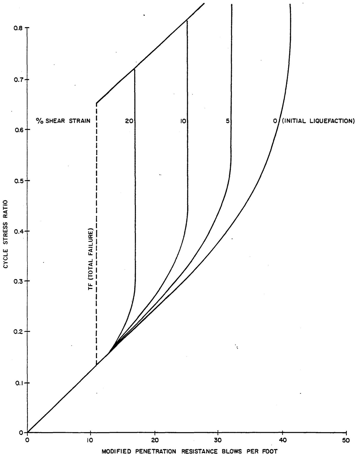
FIG. 5-59 Relationship Between Cyclic Stress Ratio Causing Different Strains and Penetration Resistance for Earthquake Magnitude = 7.0
