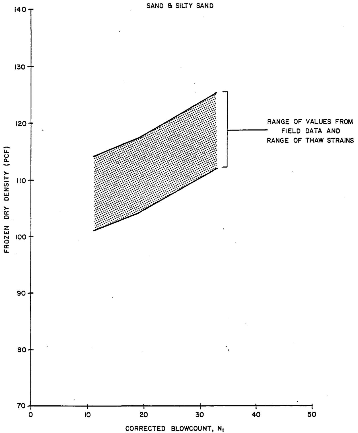
FIG. 5-68 FROZEN DRY DENSITY VERSUS CORRECTED BLOW COUNT
