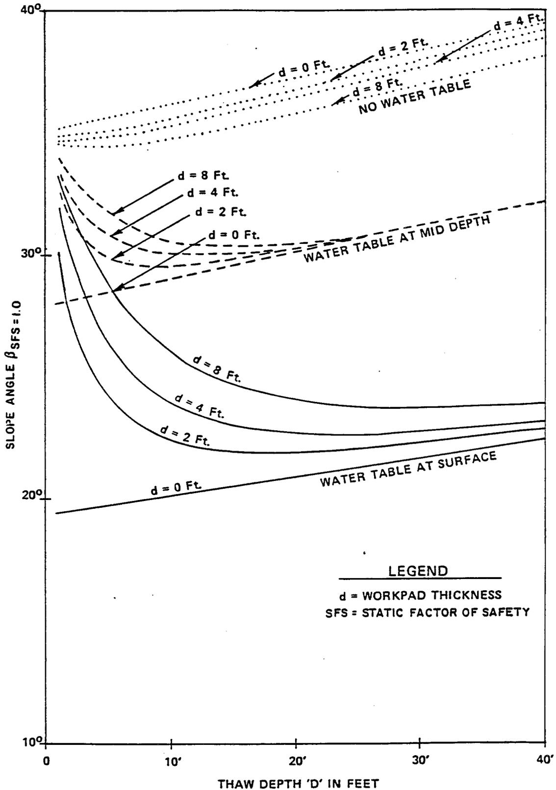
FIG. 5-16 SLOPE ANGLE FOR SFS = 1.0 vs. THAW DEPTH
