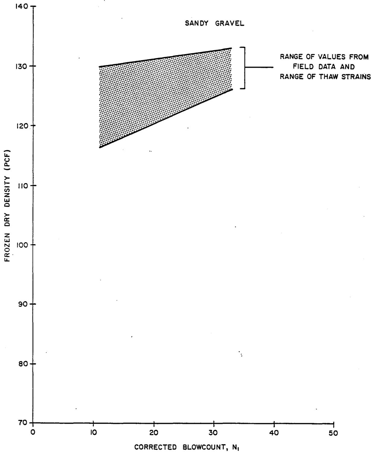
FIG. 5-66 FROZEN DRY DENSITY VERSUS CORRECTED BLOW COUNT
