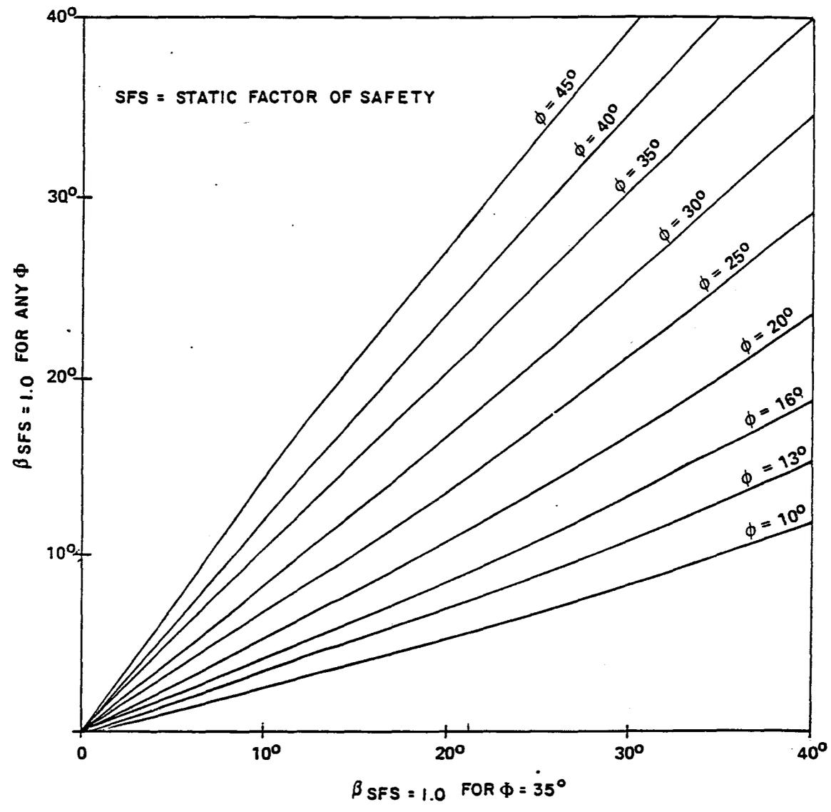
FIG. 5-21 SLOPE ANGLE FOR SFS = 1.0 FOR  $\phi = 35^\circ$ ,  $C = 0$  vs. CORRESPONDING SLOPE ANGLE FOR ANY  $\phi$
