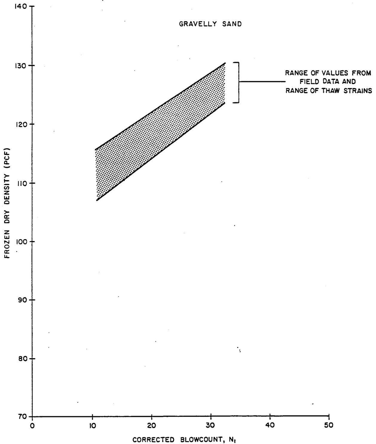
FIG. 5-65 FROZEN DRY DENSITY VERSUS CORRECTED BLOW COUNT
