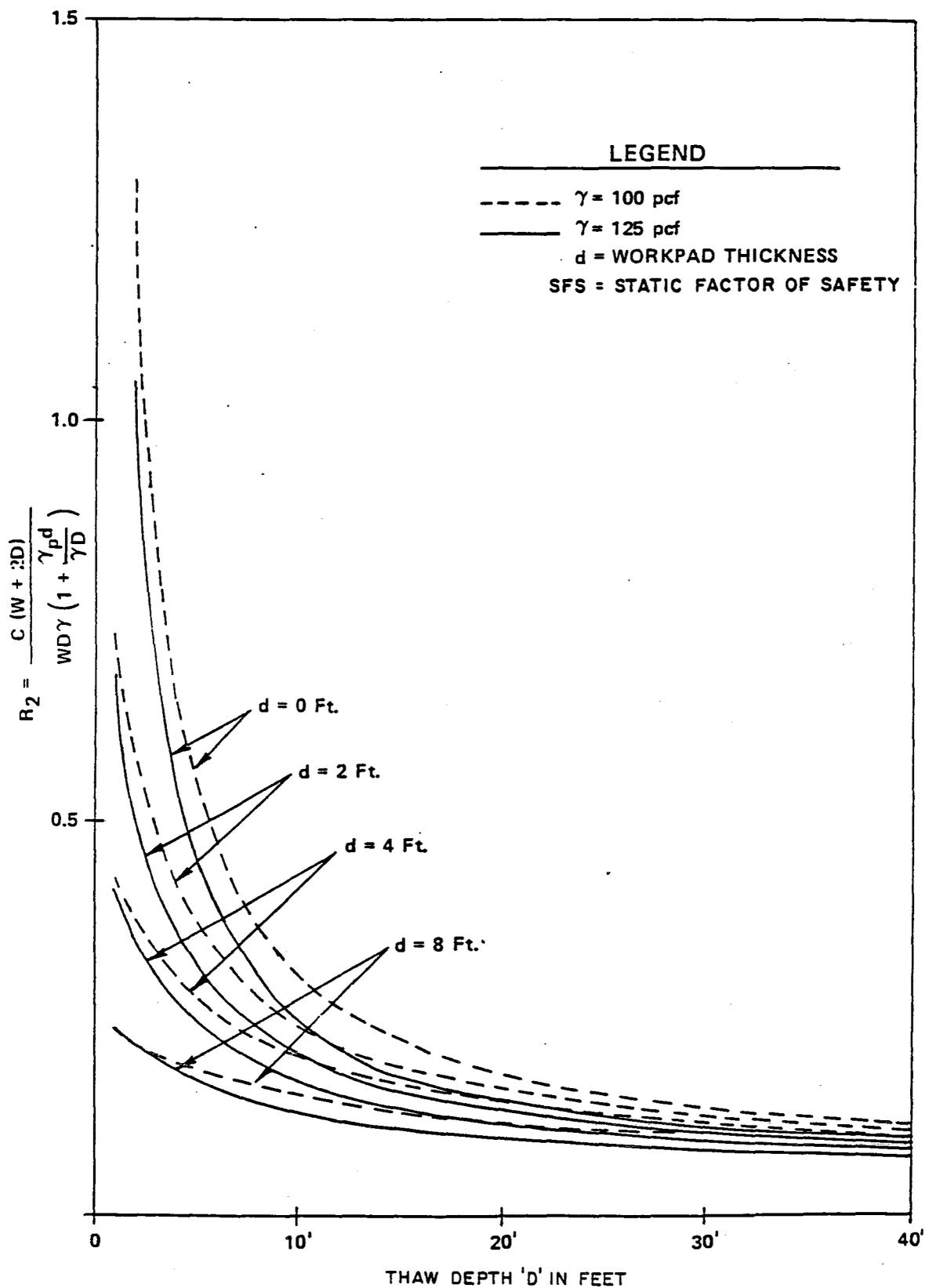
FIG. 5-20  $R_2$  (COHESION COMPONENT OF SFS) vs. DEPTH OF THAW
