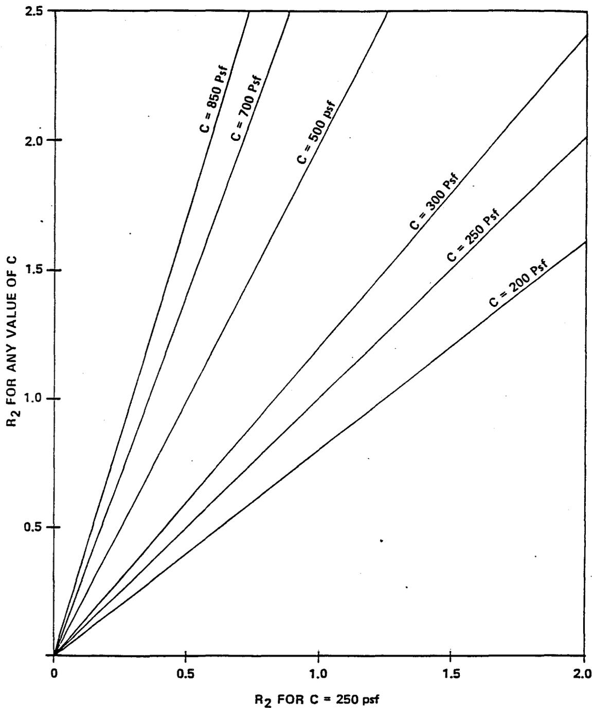
NOTE:  $R_2 = \frac{C (W + 2D)}{WD\gamma (1 + \gamma_p d / \gamma D)}$
