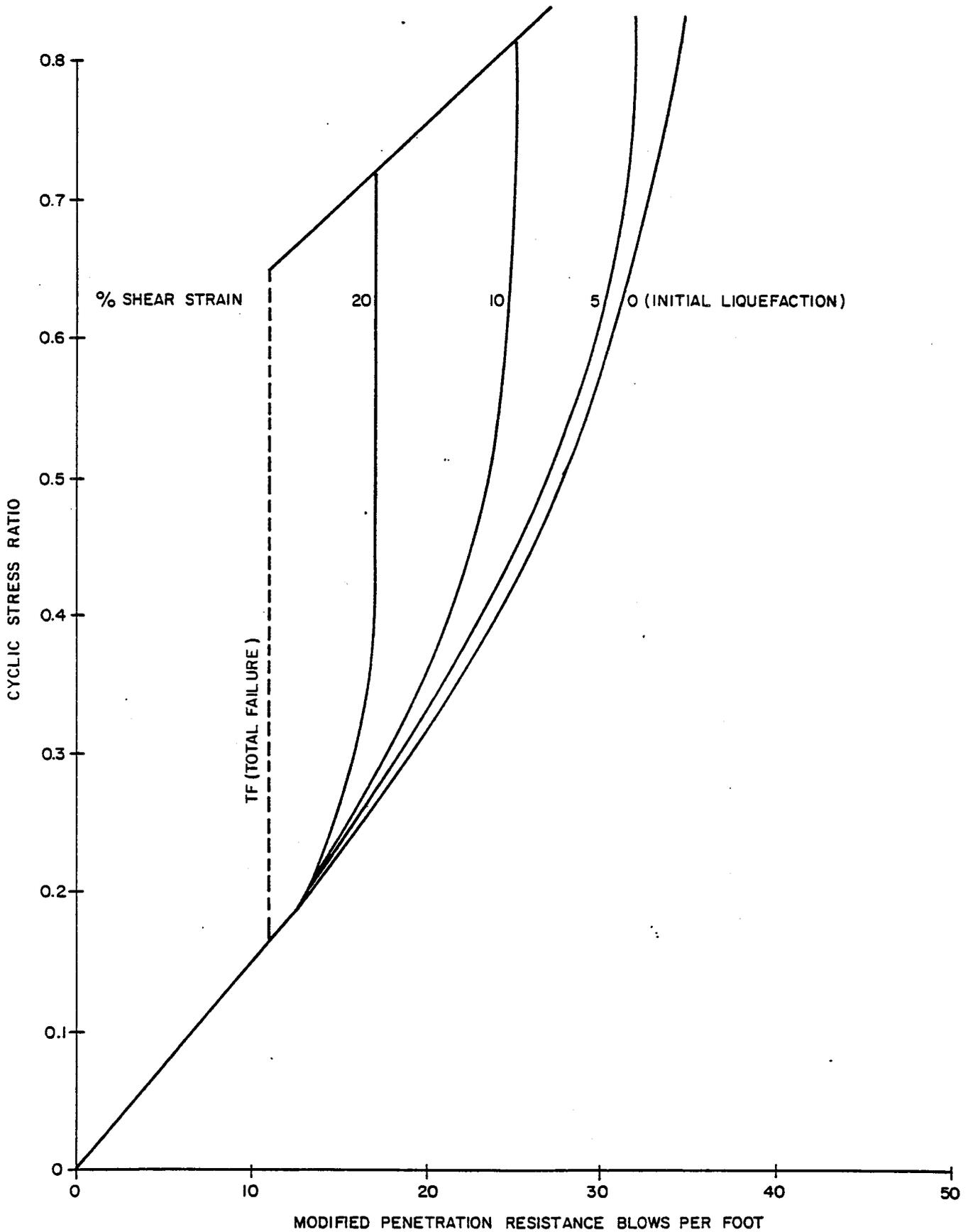
FIG. 5-60 Relationship Between Cyclic Stress Ratio Causing Different Strains and Penetration Resistance for Earthquake Magnitude = 5.5
