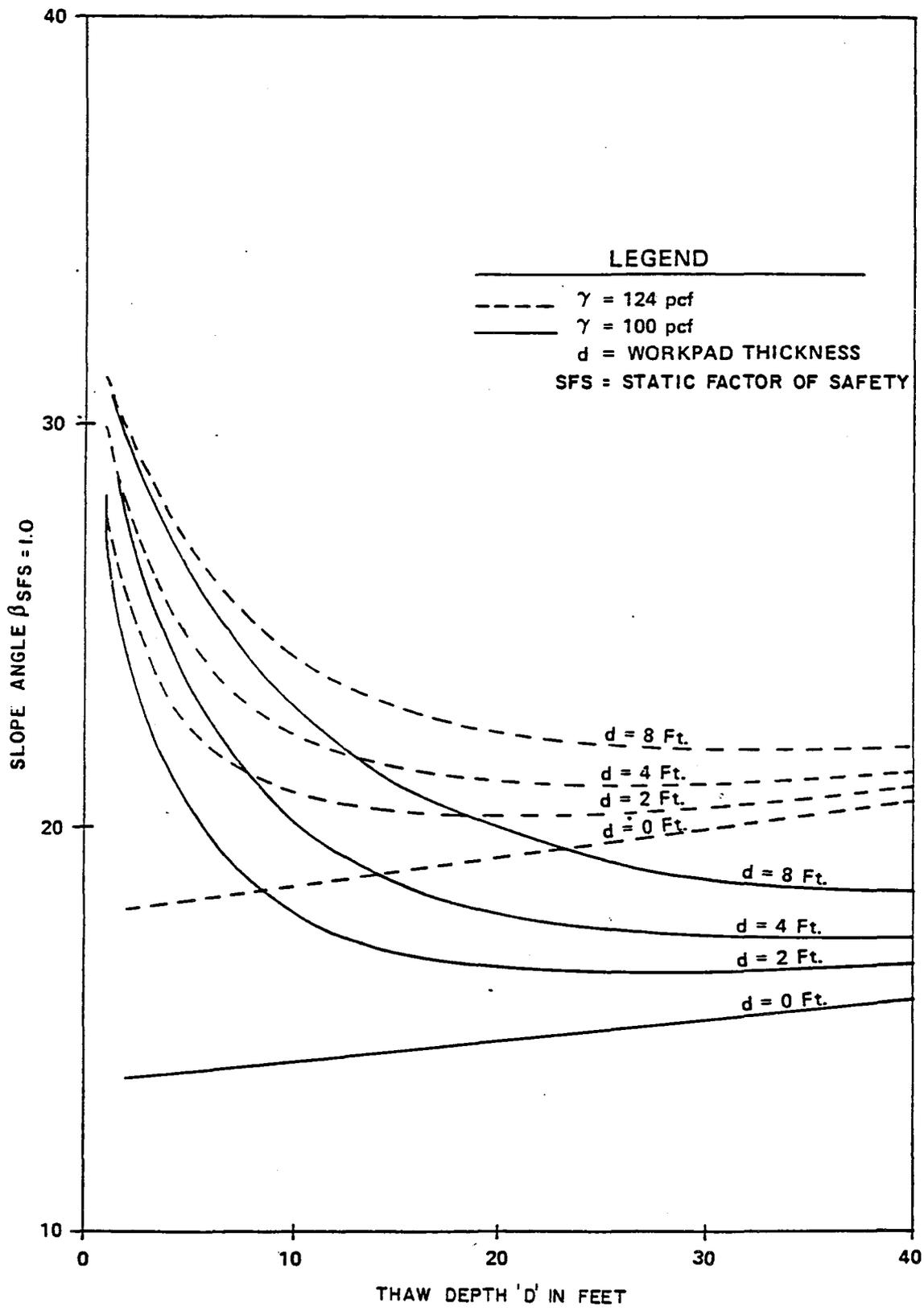
FIG. 5-19 SLOPE ANGLE FOR SFS=1.0 vs. THAW DEPTH
