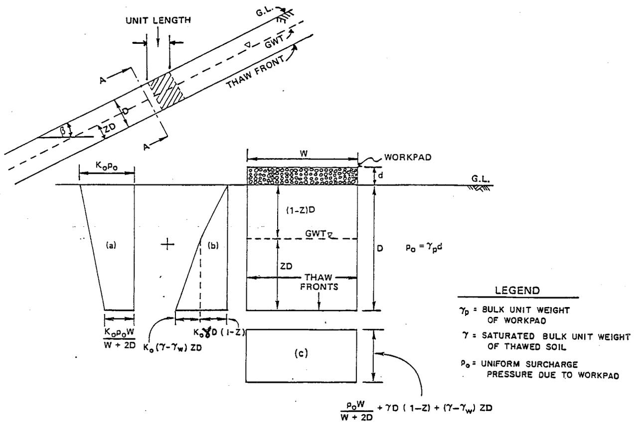
$$SFS = \frac{1}{1 + X} \left[ \left\langle \frac{K_o D}{W} \left( 1 - \frac{\gamma_w}{\gamma} Z^2 \right) + \left( 1 - \frac{\gamma_w}{\gamma} Z \right) \right\rangle + \left( \frac{X}{W/D + 2} \right) \left\langle 2K_o \left( 1 + \frac{D}{W} \right) + \frac{W}{D} \right\rangle \right] \frac{\tan \phi}{\tan \beta}$$
