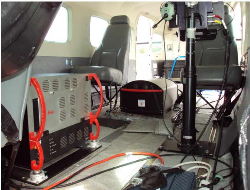
Source: Alaska Division of Geological & Geophysical Surveys A Cessna Caravan loaded with lidar gear.
