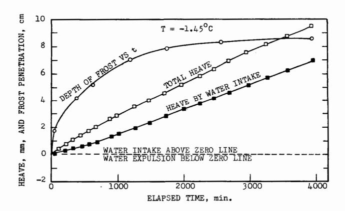
Fig. 2 - Frost penetration and heave rate measurements at 1 kg/cm<sup>2</sup> for Soil No. 2
