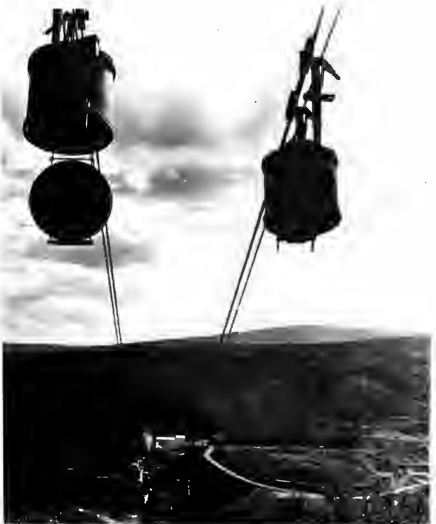
Ore buckets carry material from open pit to the mill at the Cassiar Asbestos mine, Clinton Creek (Yukon government)
