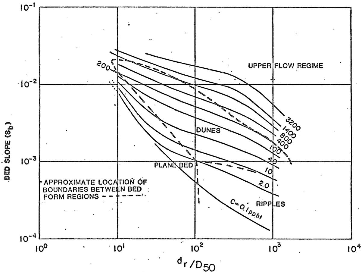
SLOPE -  $d_r/D_{50}$  RELATION FOR FLOW IN ALLUVIAL CHANNELS AT VARIOUS VALUES OF BED-LOAD CHARGE, C (AFTER COOPER, PETERSON BLENCH REFERENCE)
