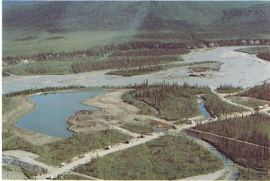
Plate 29. M.S. 101-1 located in and adjacent to the Middle Fork Koyukuk River in A.S. 101, Section 5. The southern portion of the site has clear ponded water while the northern aliquot (right side of photo at end of access road) is nearly all submerged by flowing water. The work pad intersects armored spur dikes. JFWAT photo 579-13 by J. Gustafson; June 1976.
