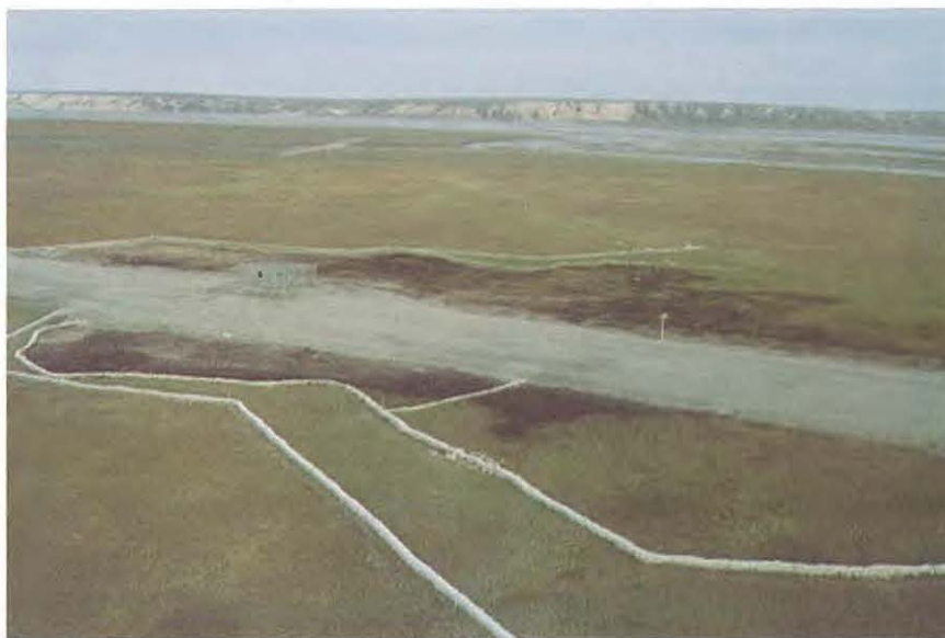
Plate 13. Crude oil spill on wet-meadow tundra (HQ) in A.S. 133, Section 6. Sorbent and containment booms are in place around the spill area. The fenced structure (left portion of the pad) is Valve #7 which was the source of the spill. View is east toward the Sagavanirktok River. JFWAT photo 976-10 by J. Gustafson; August, 1978.
