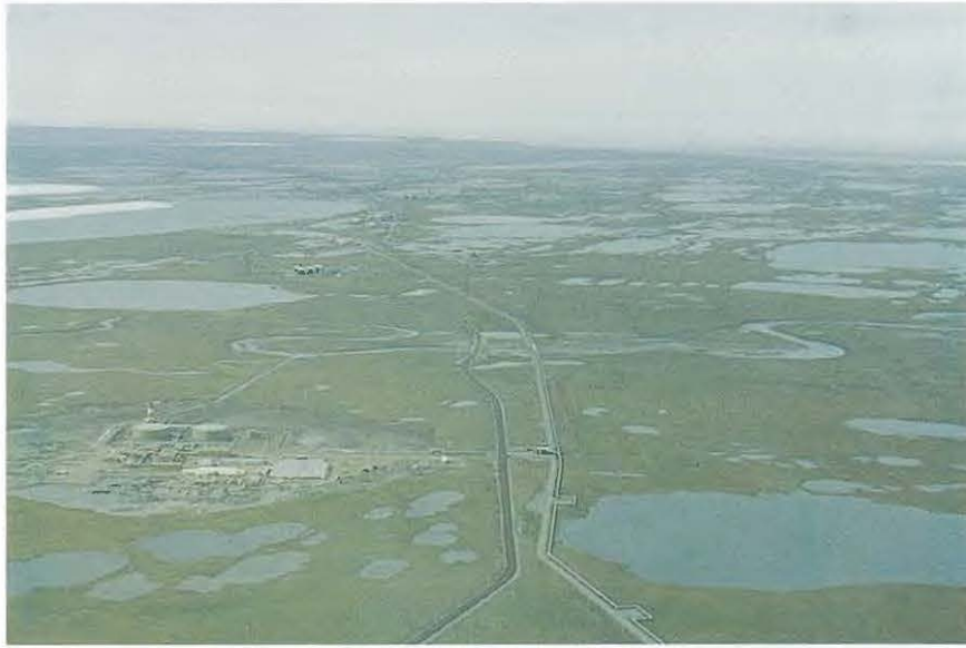
Plate 27. Pump Station 1 built in wet-meadow tundra (HQ) about four miles south of Prudhoe Bay in A.S. 138, Section 6. View is northwest. A lake of approximately 140 surface acres in size was drained so that this pump station could be constructed. JFWAT photo 868-1 by R. Hallock; July, 1977.
