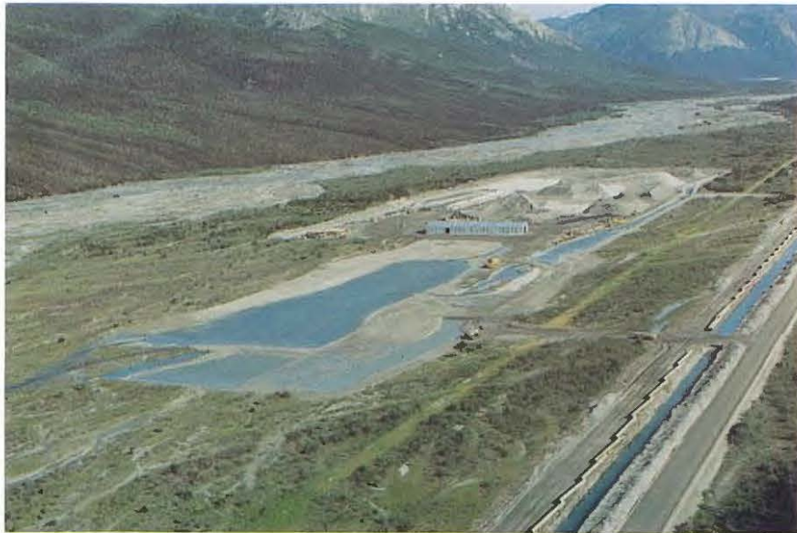
Plate 30. M.S. 106-2 located in the Dietrich River floodplain, A.S. 106, Section 5. This material site destroyed primarily riparian willow (HMQ). It was mined deep on the south end to provide overwintering habitat for fish. Open trench for below-ground pipe and the Haul Road can be seen on the right side of the photo. JFWAT photo 580-14 by J. Gustafson; June, 1976.
