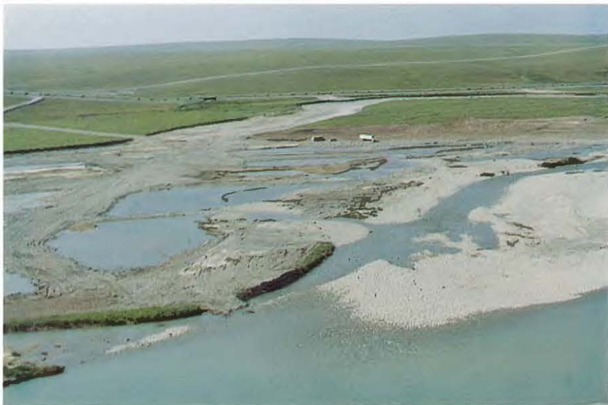
Plate 34. Material site located in the floodplain of the Sagavanirktok River, Section 6. View is west toward the pipeline and Haul Road. Note access road to site. Riparian willow (HMQ) and unvegetated floodplain (LQ) habitats were most affected by this mining operation. Over 5,200 surface acres were mined in the Sagavanirktok floodplain. JFWAT photo 897-9 by M. Haddix; July, 1977.
