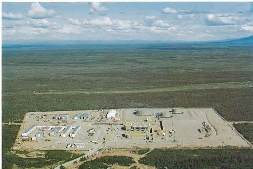
Plate 28. Pump Station 9 which was constructed in spruce-deciduous woodland (HMQ) and spruce woodland (LMQ) in A.S. 44, Section 2. View is east. The work pad joins the north and south sides of the site (about 43 acres). JFWAT photo 818-10 by E. Westman; June, 1977.
