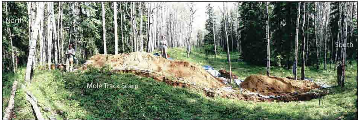
Figure 14. The "mole track" scarp on the Dot "T" Johnson fault at trench I viewed looking east. This section of the scarp exhibits a distinct "mole track" morphology indicative of a near-surface thrust wedge at the tip of a shallow-dipping thrust fault.
