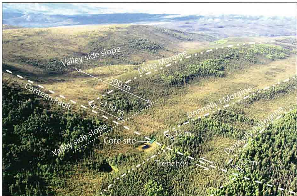
Figure 8. Oblique air photograph looking to the northwest of Donnelly- and Delta-age moraines offset by the Canteen fault on the west side of the Little Gerstle River valley. The pond core site (green box) and trench (yellow box) are shown. Left-lateral offsets of the Donnelly moraines (32 m) were measured with a surveying tape in the field. Offset of the Delta moraine (~110 m) was determined from a GPS survey. The offset of the side slope of the river valley (~500 m) was estimated from a vertical air photo.
