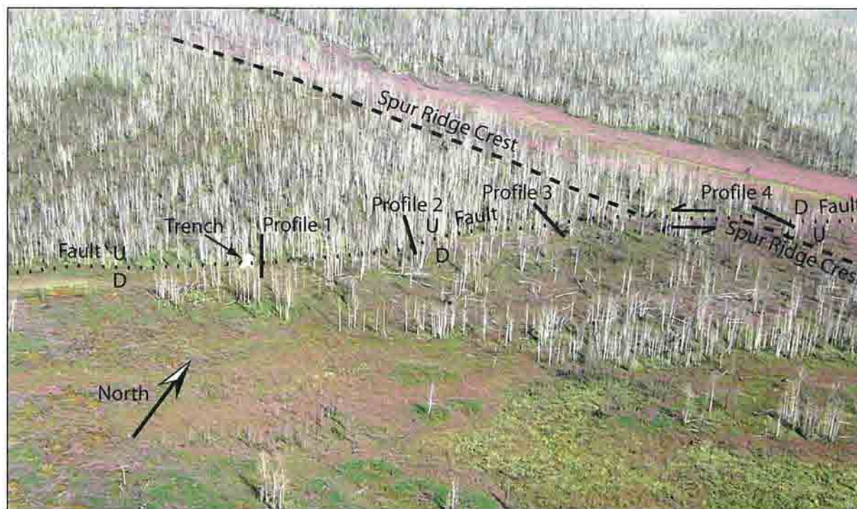
Figure 5. Oblique aerial photograph of the Billy Creek fault at the trench site. The northeast-trending fault forms a prominent scarp about 2 to 3 m high marked by a vegetation contrast between trees to the northwest and tundra to the southeast, probably reflecting differences in depth to shallow groundwater across the fault. The trench (covered by a white weather shelter) is in the middle left half of the photograph. The locations of scarp profiles shown in figure 6 are shown on the photo. This area burned in a wildfire in 2004. The photograph was taken in 2007. U = upthrown side of fault; D = downthrown side of fault.
