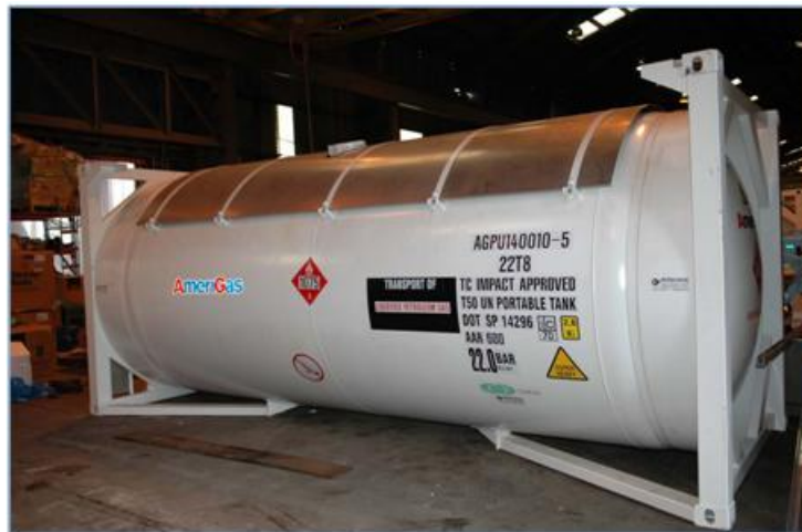
Figure 9.1. ISO Container for Propane Transportation
