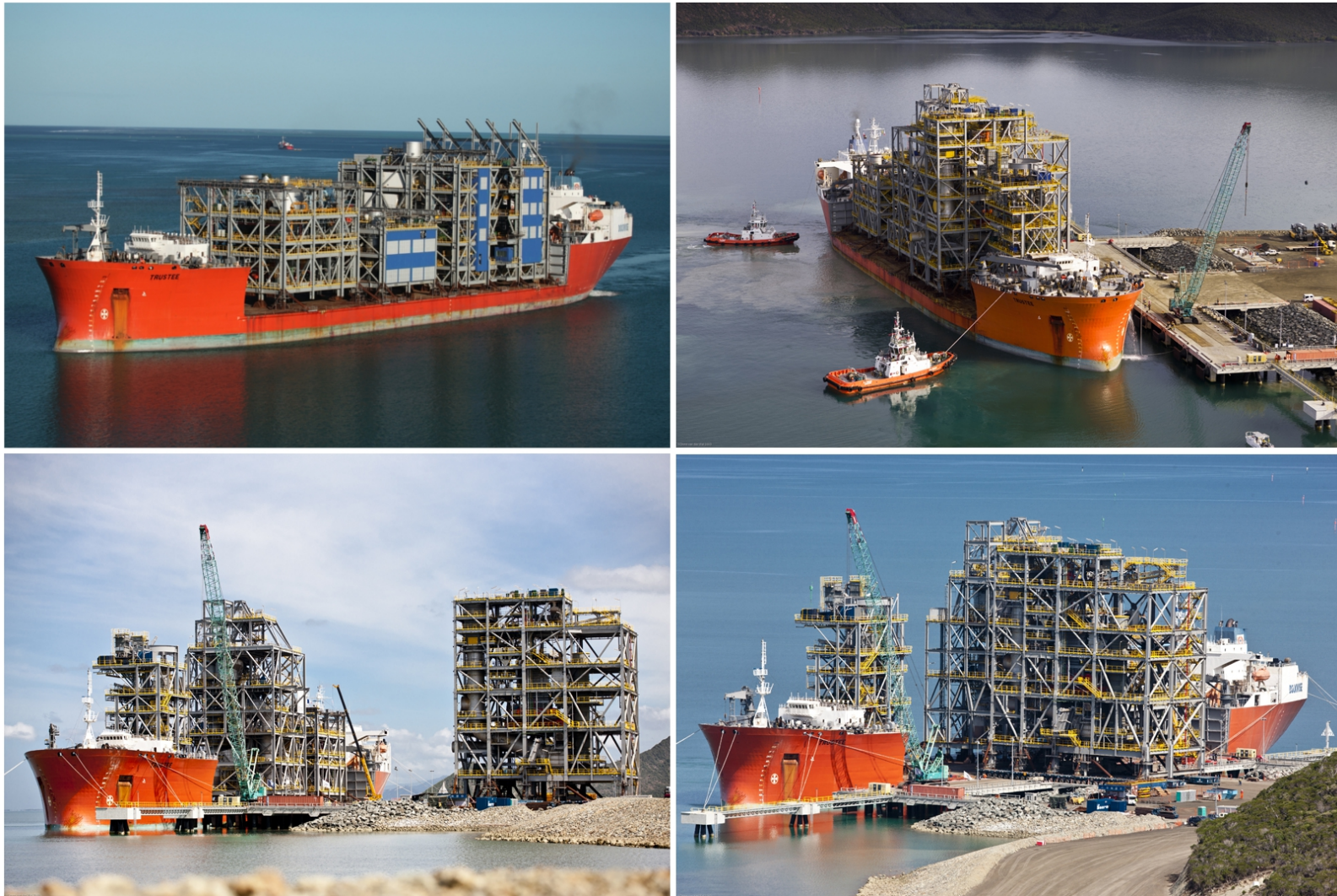
Figure 7-4: Xstrata's Koniambo Module Unloading at Site [10]
