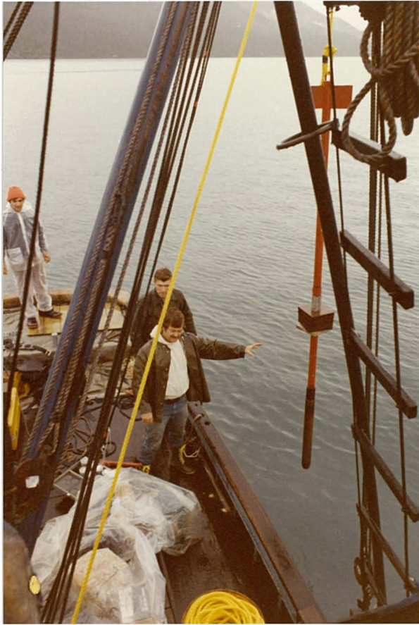
BOTTOM CORE SAMPLING DEVICE CAPABLE OF TAKING FIVE FEET OF OVERBURDEN SAMPLE
