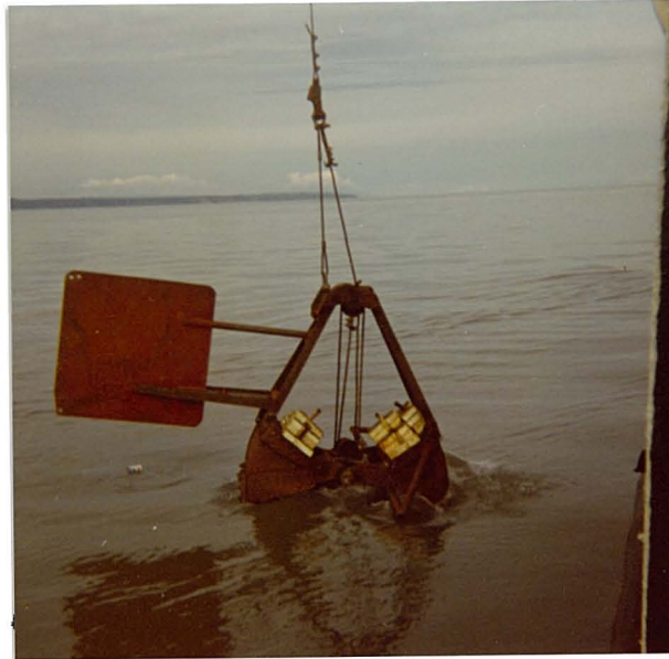
CLAM-SHELL GRAB SAMPLING EQUIPMENT SPECIFICALLY DESIGNED TO OPERATE IN COOK INLET
