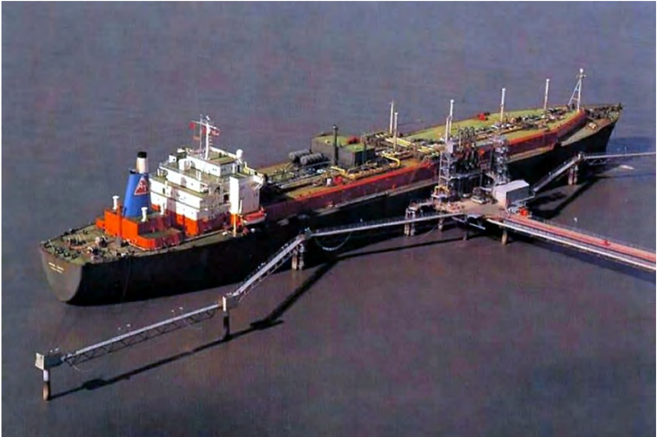
The Arctic Tokyo, shown here at the Nikiski dock, was one of two identical ships built for the startup of LNG exports from Alaska's Cook Inlet to Japan in 1969. They were the first LNG carriers known to suffer sloshing damage. The vessels were later replaced by larger models and sold off.
