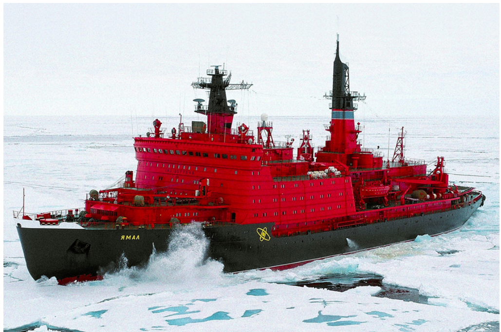
The nuclear-powered Russian icebreaker Yamal is 490 feet long with a beam of almost 100 feet. The 23,455-ton vessel was commissioned a decade ago.
