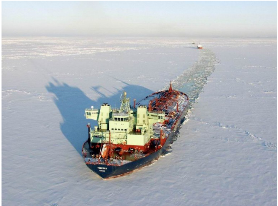
The Tempera , built a decade ago in Japan, was the first double-acting tanker ever launched. It can handle several feet of ice without the need for icebreaker assistance. It operates mainly in the Baltic Sea, carrying Russian crude to Finland.
