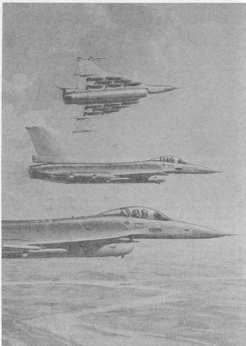
Artist's concept of the proposed advanced F-16XL in typical air-to-air and air-to-ground loadings.
