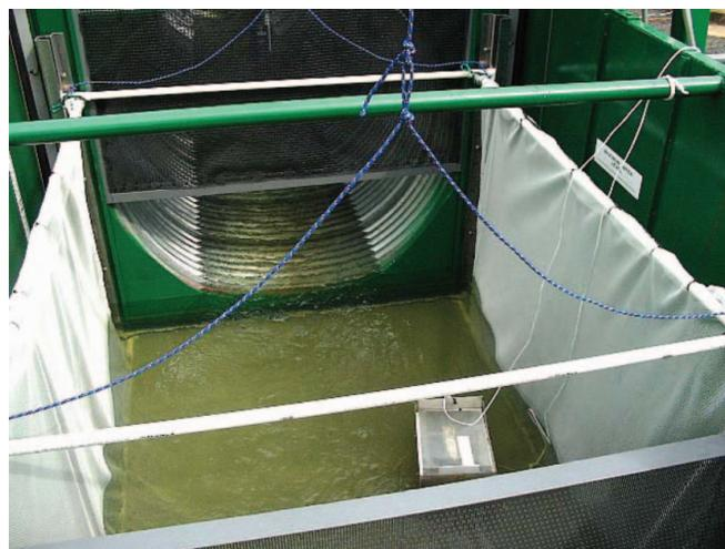
FIGURE 2. Photograph of the culvert emptying into the TW tank and associated net-pen. The net-pen is 1.83 m wide. [Figure available online in color.]
