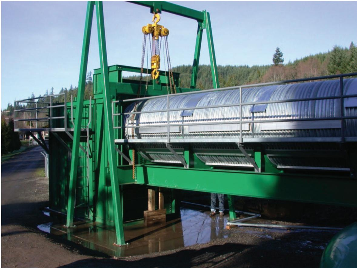
FIGURE 1. Photograph of the culvert test bed showing the culvert barrel and TW tank. The winch assembly is used to adjust the slope of the 1.83-m-diameter culvert barrel. The distance between posts in the railing is 3.05 m. [Figure available online in color.]
