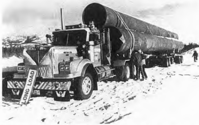
Self-Steering rear assembly of a four-axle tractor-trailer loaded with 23-m (76-ft.) lengths of pipe for test runs along the Alaska Highway.
