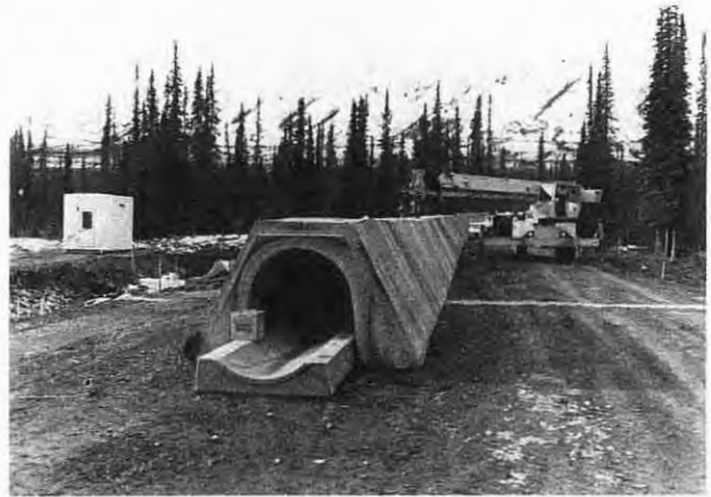
Experimental pipe installation in aboveground concrete restrained mode at Quill Creek test facility in Yukon. The pipe is placed on an insulated workpad and covered by precast concrete for protection and to provide restraint of the pipe against vertical and horizontal movements due to temperature and pressure changes.
