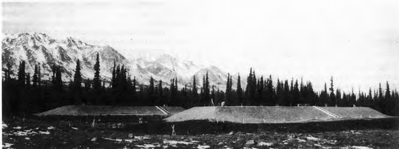
At the Quill Creek test facility, undertaken by Foothills (South Yukon) Ltd. to determine the feasibility of constructing and operating a pipeline in areas of discontinuous permafrost, pipe is installed in embankments that measure approximately 3.3 metres (10 feet) above the ground. The embankment mode consists of a gravel pad on which an insulation bed and pipe are laid and then covered with gravel. For the purposes of testing thaw settlement, pipe is also buried in the conventional manner.
