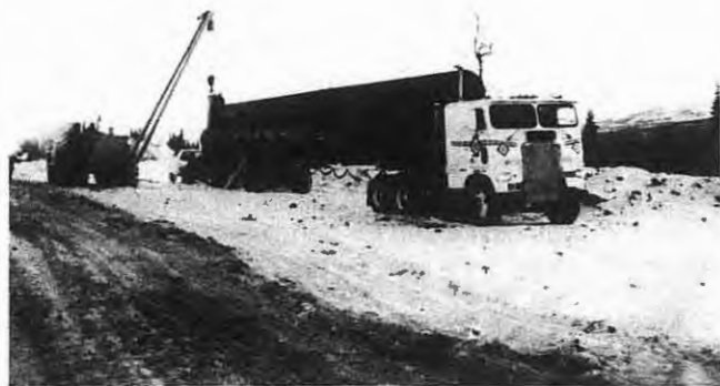
On a successful test drive from Edmonton, a specially designed tractor-trailer unit, which is capable of tracking automatically from the rear, arrives at the Quill Creek test facility in Yukon. The trip was made to test the new vehicle's ability to carry long joints of pipe around sharp corners such as those along the Alaska Highway.
