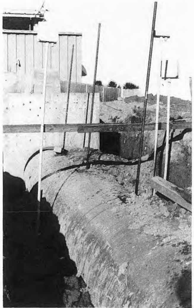
CALGARY FROST HEAVE TEST SITE—Illustrating insulated pipe in ditch, attached level indicator rods and thermistors for measuring ground and pipe temperatures—September 22, 1978.
