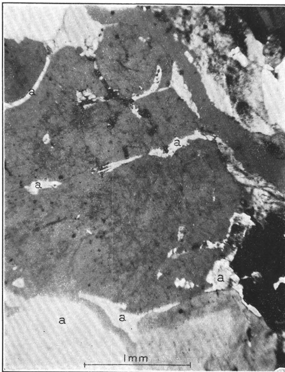
C. WISPS OF RESIDUAL ALBITE (a) IN QUARTZ WHICH IS REPLACING IT All the albite shown extinguishes simultaneously.
