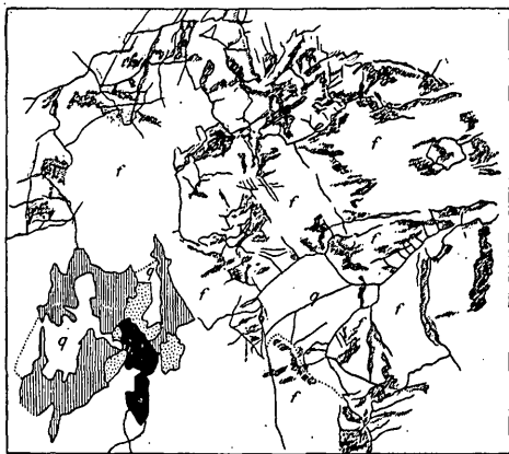
FIG. 2.—Minerals in thin section (3.76 by 4.23 millimeters = 0.15 by 0.17 inch) of biotite granite from High Isle in Knox County, showing "sap." The ramifications of "sap" (limonite stain) across and around feldspar and quartz particles (marked f and q ) are independent of the biotite and magnetite particles. Fine-lined parts are biotite; fine-dotted areas are titanite; large black masses are magnetite. Some of the borders of quartz particles are shown by dotted lines.
