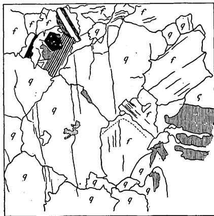
FIG. 1.—Outlines of minerals, in thin section (four-fiftieths inch square) of biotite-muscovite granite from Weskeag quarry, near Pleasant Beach, South Thomaston, showing parallel rift cracks crossing quartz and feldspar particles (marked q and f ). The finely shaded parts are muscovite and biotite; the banded area is oligoclase. The black pentagonal area is a crystal of garnet.
