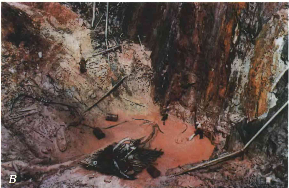
Figure 19. Saprolite-gold system, kaolinite-bearing surficial deposit, Kilometro 88, Estado Bolívar. A , Sidewall of prospect pit showing relict foliation in saprolitic metavolcanic sequence. Photograph by Floyd Gray. B , Kaolinite zones in gold prospect pit; lines are from hydraulic system used in mining saprolite-kaolinite. Photograph by Dennis Cox.
