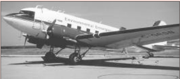
The specially equipped DC-3 propeller-driven aircraft can fly low and slow providing a stable platform for the sophisticated remote sensing equipment. Photo courtesy Environment Canada
