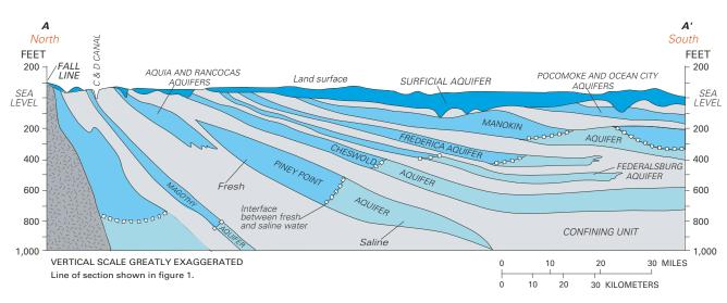
Figure 2. Sediments underlying the Delmarva Peninsula form an alternating series of confined aquifers and associated confining units, overlain by an extensive surficial aquifer that is under water-table conditions (modified from Shedlock and others, 1999).
