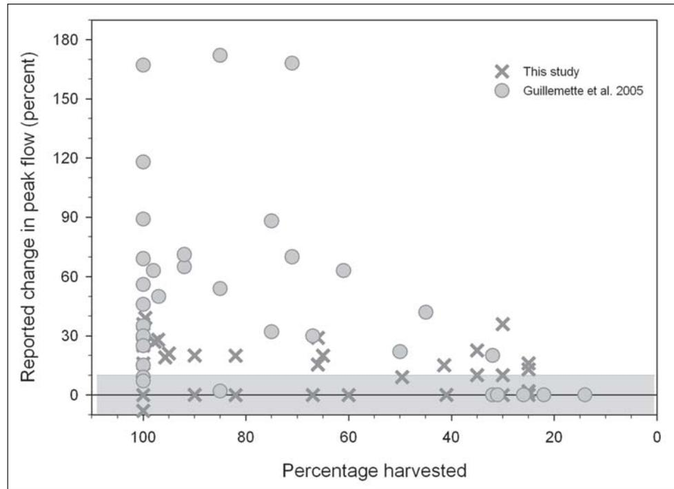
Figure 11—Reported changes to peak flow from worldwide studies, after Guillemette et al. 2005. Gray shading around zero indicates limit of detection ( $\pm 10$  percent).
