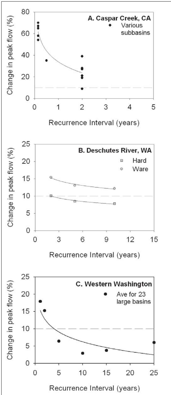
Figure 6—Reported changes in peak flow for California and Washington watersheds. Each point represents a published value for percentage increase in peak flow after harvest relative to the return period of the control watershed for (A) subbasins of Caspar Creek, California, (B) modeled basins of Deschutes River, Washington, and (C) average values of 23 large basins in western Washington. Dashed horizontal line indicates the 10-percent detection limit.
