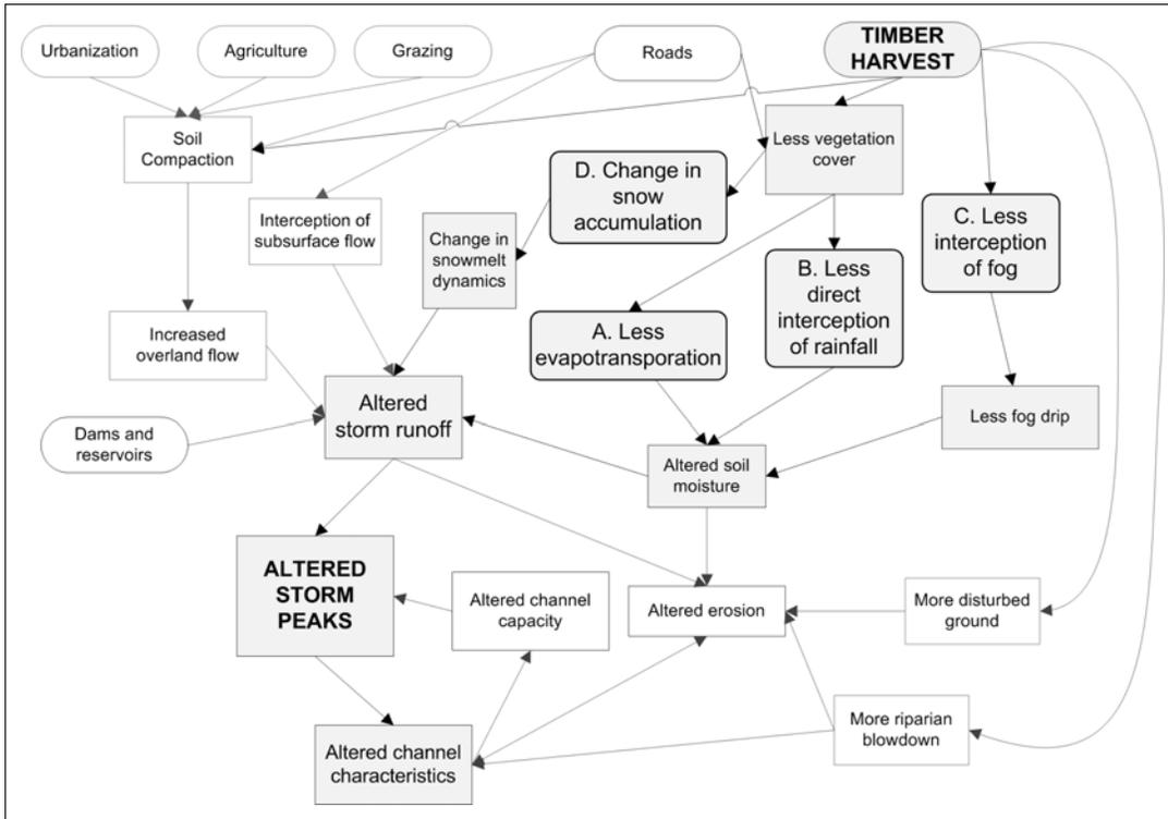
Figure 1—A process model of the relation between land use practices and altered storm peaks (after Ziemer 1998). Shading indicates processes considered in this report; A through D indicate boxes shown in figure 2.
