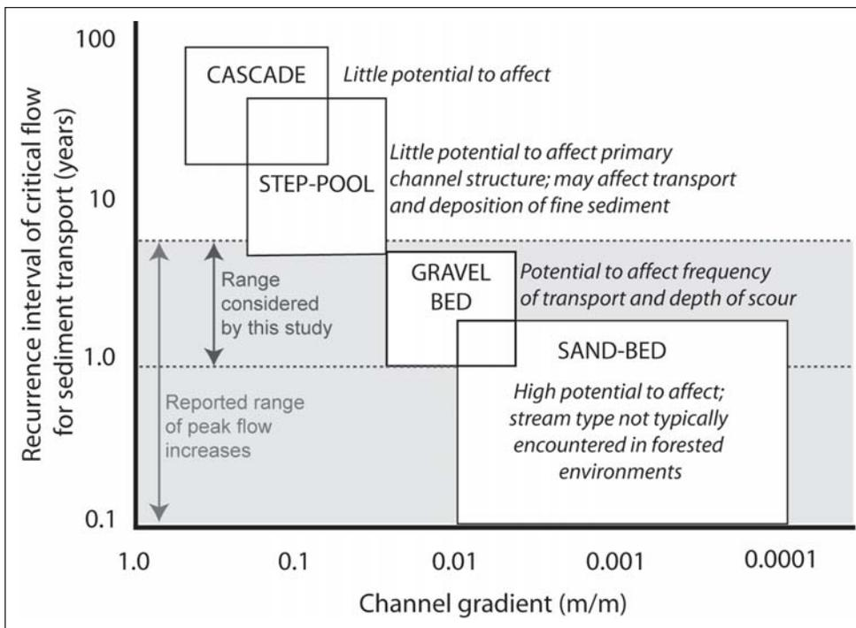
Figure 13—Domains for initiation of bedload sediment transport as a function of channel type (Grant et al. 1990, Montgomery and Buffington 1997) and recurrence interval (Andrews 1984, Grant et al. 1990, Pickup and Warner 1976, Topping et al. 2000a, 2000b, Wohl 2000).
