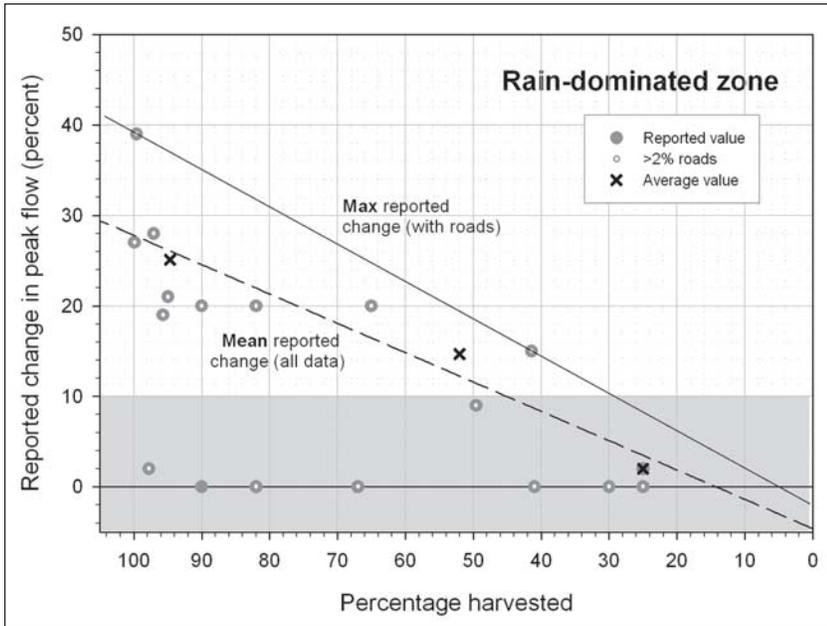
Figure 9—Peak flow response to harvest in the rain-dominated hydrologic zone. Solid line represents maximum values reported and includes the influence of roads. Dashed line is a linear fit through the average values from figure 8c, and represents the mean reported change for all data. Gray shading around zero indicates limit of detection ( $\pm 10$  percent).
